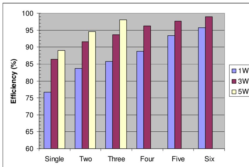
Fig. 1 Efficiency data of the SP6134HVLED evaluation board
