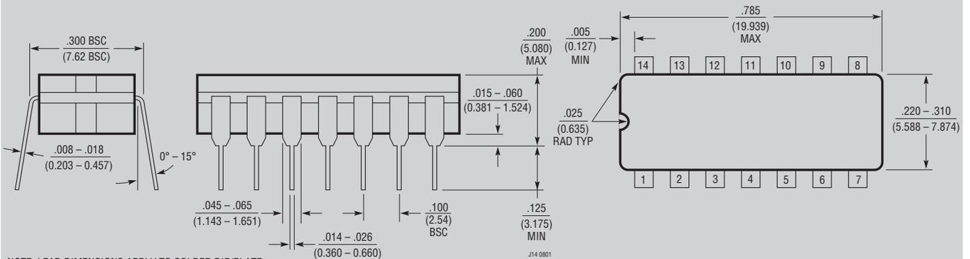
NOTE: LEAD DIMENSIONS APPLY TO SOLDER DIP/PLATE
