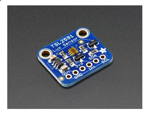
When the future is dazzlingly-bright, this ultra-high-range luminosity sensor will help you measure it. The TSL2591 luminosity sensor is an advanced digital light sensor, ideal for use in a wide range of light situations. Compared to low cost CdS cells, this sensor is more precise, allowing for exact lux calculations and can be configured for different gain/timing ranges to detect light ranges from up to 188uLux up to 88,000 Lux on the fly.
