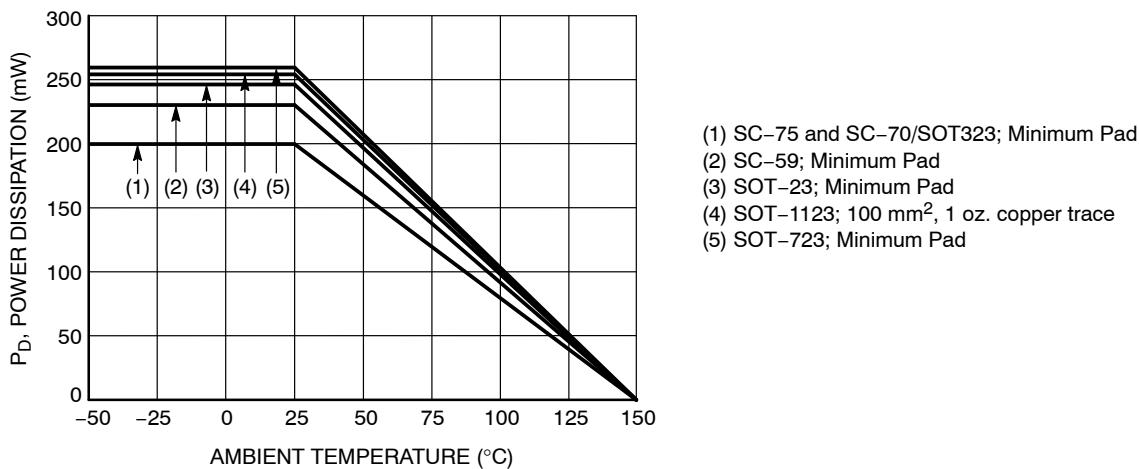
**Figure 1. Derating Curve**
