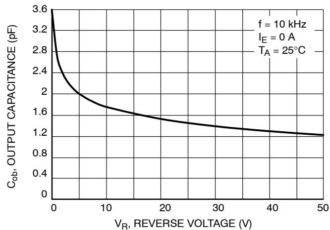
Figure 4. Output Capacitance
