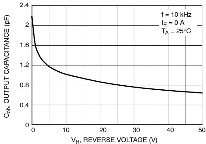
Figure 9. Output Capacitance
