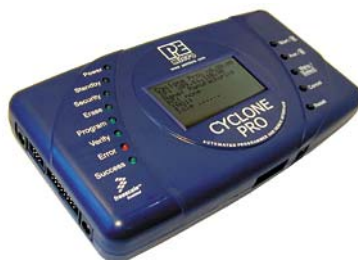
Figure 10-2: P&E's Cyclone PRO
