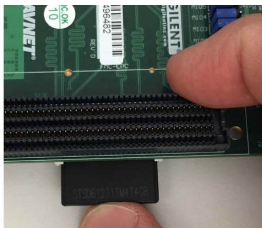
Figure 3. Inserting the SD card into the ZedBoard.
