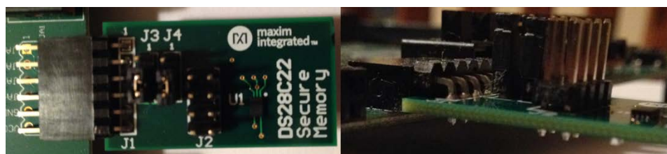
Figure 2. Pmod™ connector alignment.
