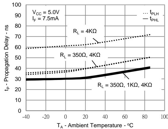
Figure 9: Typical Propagation Delay vs. Ambient Temperature
