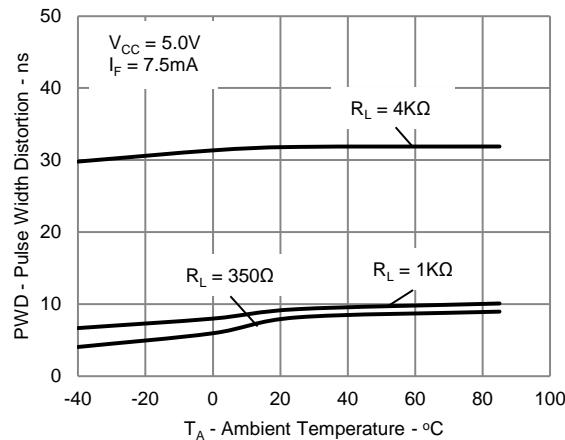
Figure 10: Typical Pulse Width Distortion vs. Ambient Temperature
