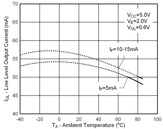
Figure 7: Typical Low Level Output Current vs. temperature
