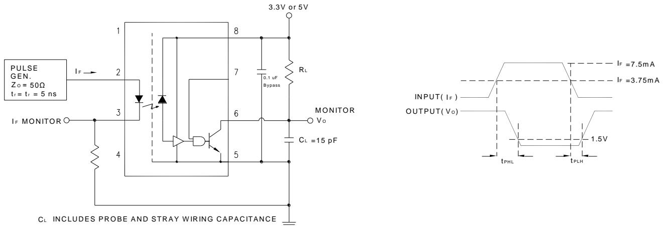
Figure 1: Test Circuit for  $t_{PHL}$  and  $t_{PLH}$
