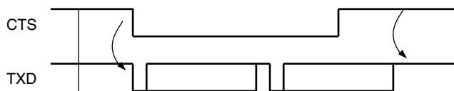
Figure 40-28. Transmitter Behavior when Operating with Hardware Handshaking
