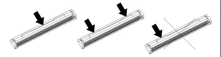
◆ Release the actuator to remove the FPC.
