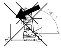
Operate the actuator only as instructed. Do not attempt to dislodge the open actuator as shown below.
