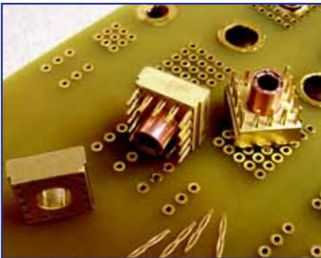
The RADSOK® PowerBlok™ provides a high current single-point connection to the PCB with the proven reliability of compliant pin signals. The PowerBlok™ is designed to bring up to 70 Amperes to the board, utilizing our custom 3.0mm RADSOK® design. The compliant pins are press-fit into the board to secure a solid connection and even flow.
