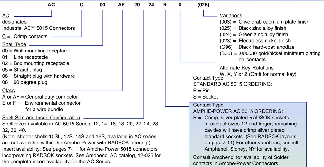
\*\* Amphe-Power 5015 Connectors are based on the AC Threaded Series from Amphenol which incorporates 5015 contact arrangements. Within the AC family a reverse bayonet style is also offered, but the bayonet style is not currently offered with RADSOK sockets. See Amphenol catalog 12-025 for more information on the AC connector family.
