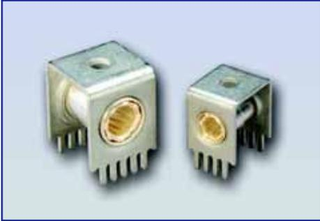
The RADSOK® PGY™ is our orthogonal card edge series. The 5.7mm PGY™ is our highest current board level product rated to 120 Amperes. The PGY™ is connected to the board through a solder reflow process. The busbar pin will mate horizontally with RADSOK® slightly above the board.
