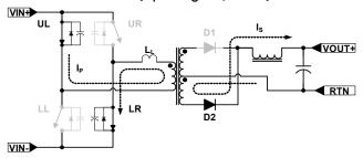
FIGURE 13. UL TO LR POWER TRANSFER CYCLE
