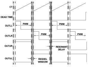
FIGURE 11. BRIDGE DRIVE SIGNAL TIMING
