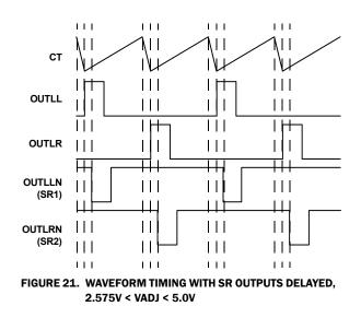
Setting VADJ to VREF/2 results in no delay on any output. The no delay voltage has a  $\pm$ 75mV tolerance window. Control voltages below the VREF/2 zero delay threshold cause the PWM outputs, OUTLL/LR, to be delayed. Control voltages greater than the VREF/2 zero delay threshold cause the SR outputs, OUTLLN/LRN, to be delayed. It should be noted that when the PWM outputs, OUTLL/LR, are delayed, the CS to output propagation delay is increased by the amount of the added delay.
