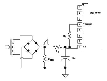
FIGURE 9. ADDING SLOPE COMPENSATION
