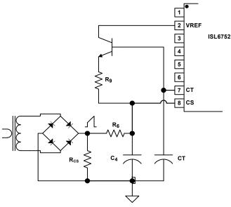
FIGURE 10. ADDING SLOPE COMPENSATION USING CT
