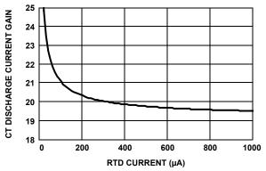
FIGURE 5. CT DISCHARGE CURRENT GAIN vs RTD CURRENT
