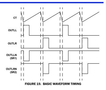
Referring to Figure 19, the SRs alternate between being both on during the free-wheeling portion of the cycle (OUTLL/LR off) and one or the other being off when OUTLL or OUTLR is on. If OUTLL is on, its corresponding SR must also be on, indicating that OUTLRN is the correct SR control signal. Likewise, if OUTLR is on, its corresponding SR must also be on, indicating that OUTLLN is the correct SR control signal.
