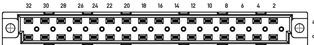
Lötanschluß 1,0 x 1,0 mm / solder terminal 1,0 x 1,0 mm
