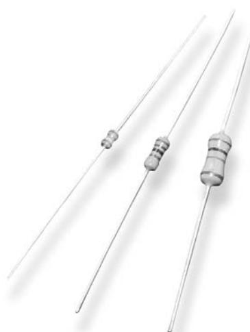
The resistive element comprises a thin film of nickel-chrome alloy evaporated onto a high thermal conductivity ceramic element. Metal end caps are force fitted to the element prior to spiralling to value. Tinned copper lead wires are welded to the end caps and the components are then coated. One coat of phenolic resin is followed by three coats of epoxy resin. All resistors are tested for value and tolerance.
