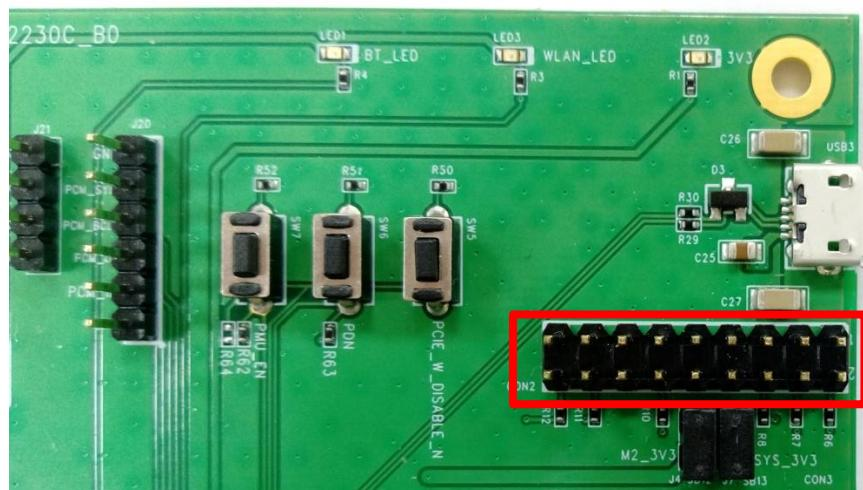
*Figure 2: DVK-SU60-2230C SDIO Pin Header*
