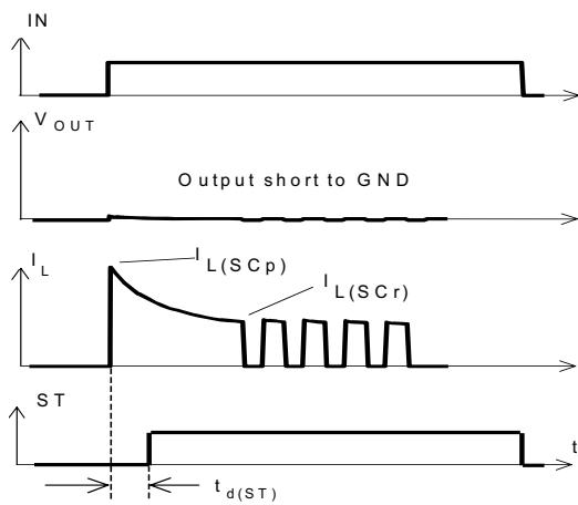
Heating up of the chip may require several milliseconds, depending on external conditions.
