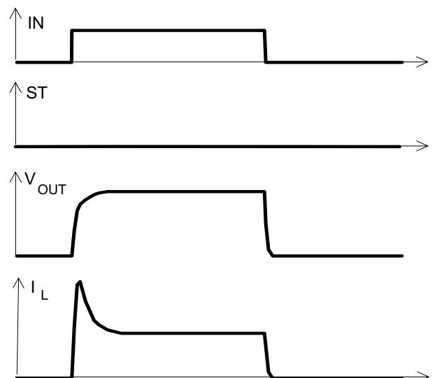
**Figure 2a:** Switching a resistive load,
