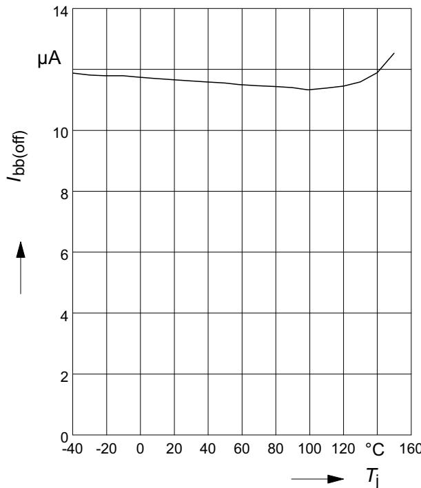
**Typ. leakage current**
