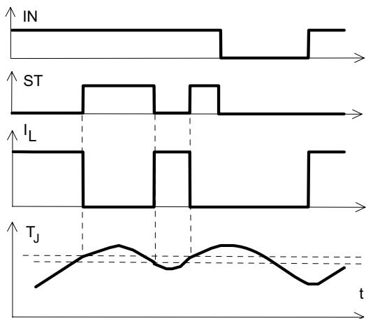
**Figure 3b:** Short circuit in on-state
