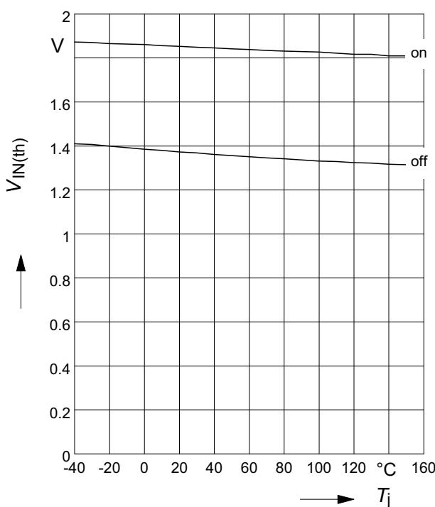
**Typ. input threshold voltage**
