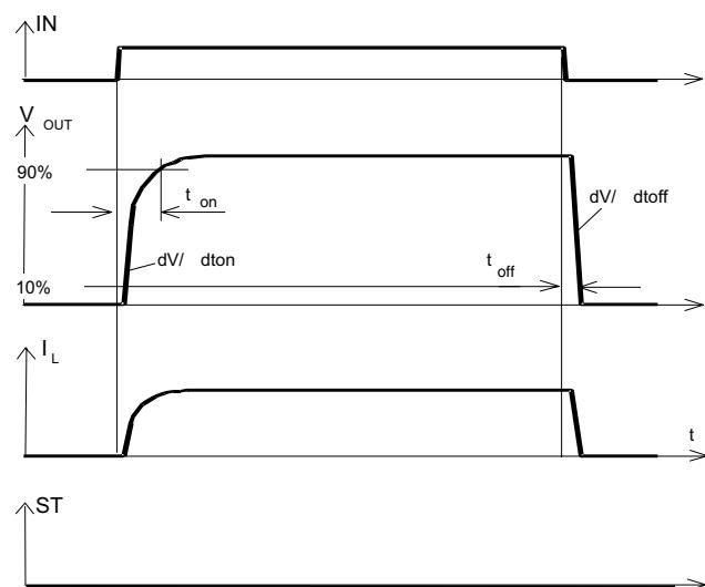
**Figure 2c:** Switching an inductive load
