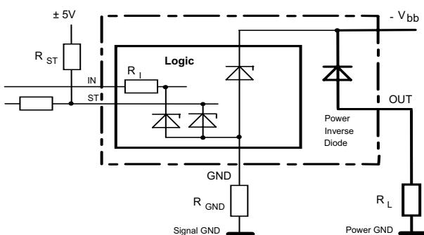
$R_{GND}=150\Omega$ ,  $R_I=3.5\text{k}\Omega \text{ typ.}$
