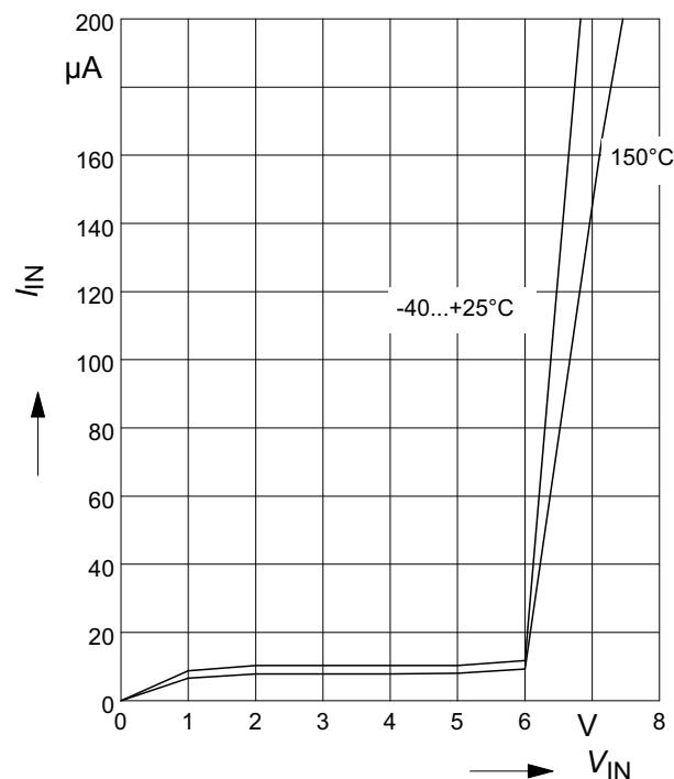
**Typ. input threshold voltage**
