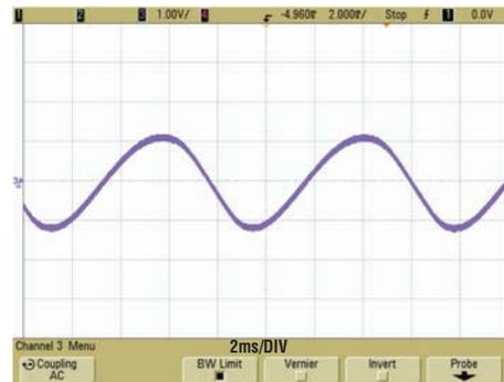
Figure 12. Output Ripple at 230VAC, 2A Load
