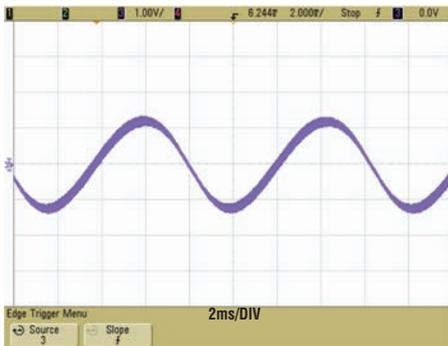
Figure 11. Output Ripple at 120VAC, 2A Load
