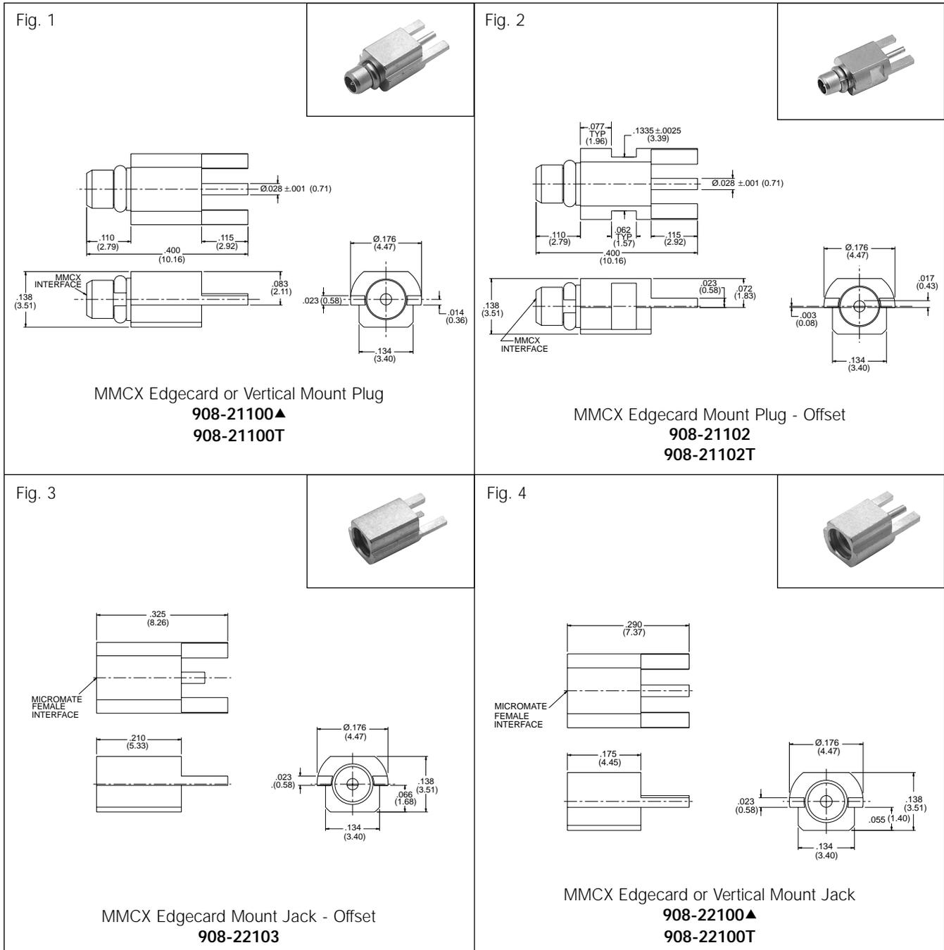
**MicroMate™ (MMCX) EDGE CARD AND PCB MOUNTS**
