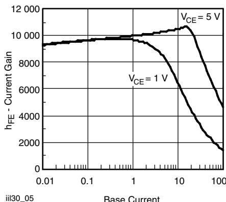
Fig. 5 -  $h_{FE}$  Current Gain vs. Base Current
