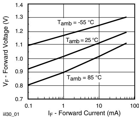
Fig. 1 - Forward Voltage vs. Forward Current
