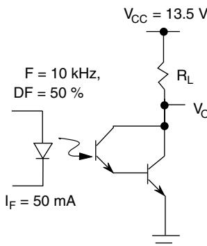
Fig. 9 - Switching Schematic
