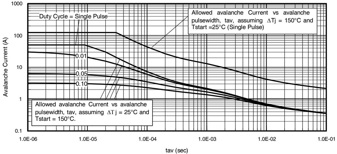
**Fig 15. Typical Avalanche Current vs. Pulse width**
