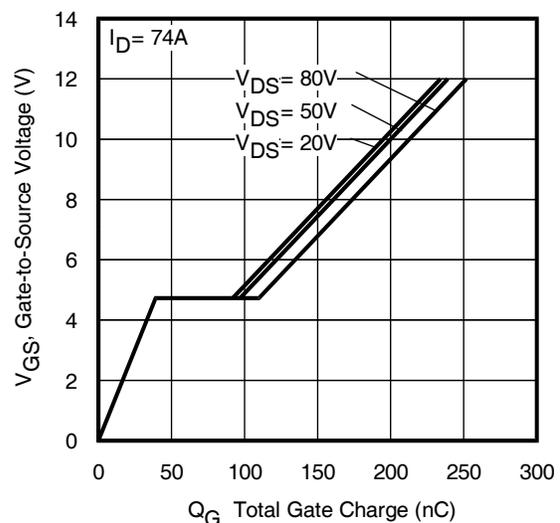
**Fig 9. Typical Gate Charge vs. Gate-to-Source Voltage**
