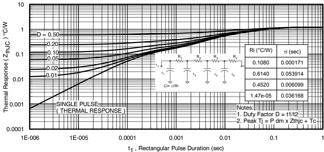
Fig 3. Maximum Effective Transient Thermal Impedance, Junction-to-Case
