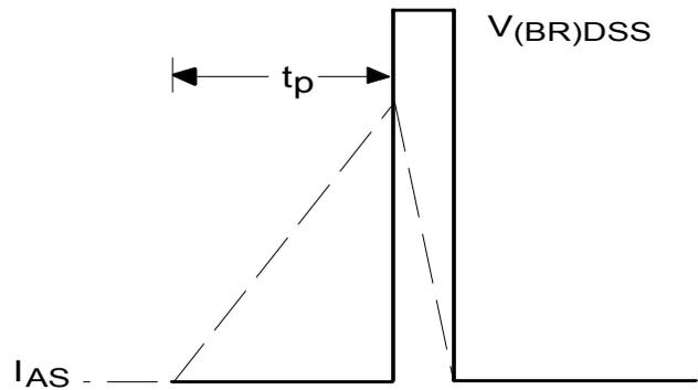
**Fig 19b.** Unclamped Inductive Waveforms
