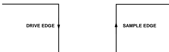
Figure 41. SPI Mode 3 SCLK Edges
