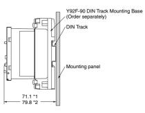
Using a PFP-50N or PFP-100N Mounting Track.
