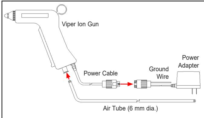
Figure 3. Installing the Viper Ion Gun
