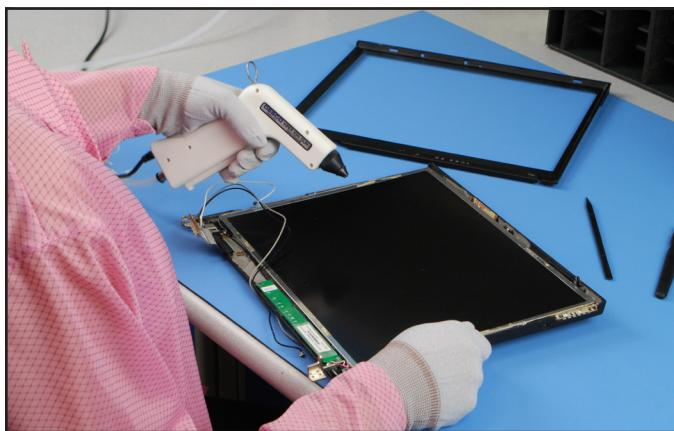
Figure 4. Using the Viper Ion Gun
