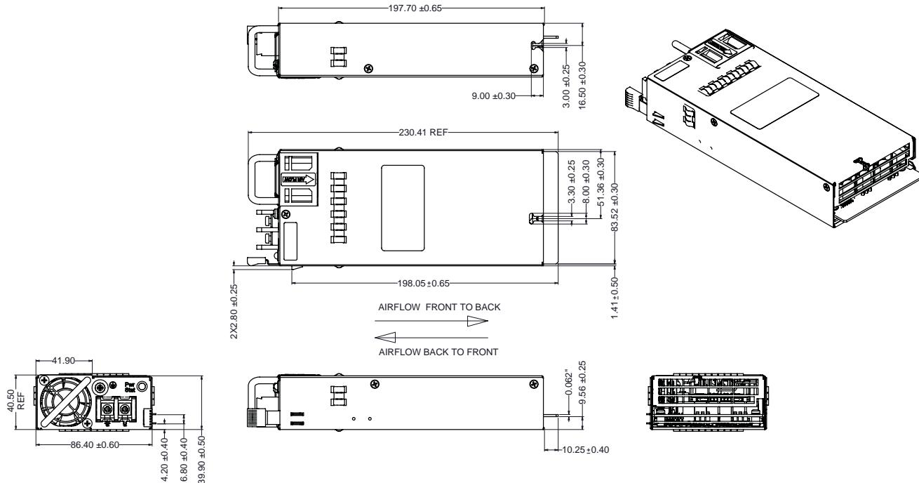
DC input connector: Terminal Block, Dinkle Enterprise: Part No. DT-7C-B14W-02
