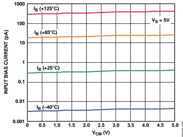
Figure 6. Input Bias Current vs. Common-Mode Voltage
