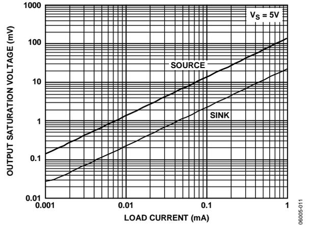
Figure 11. Output Saturation Voltage vs. Load Current
