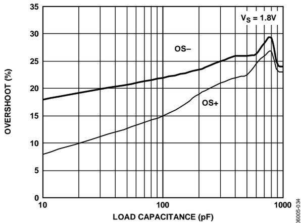
Figure 34. Small Signal Overshoot vs. Load Capacitance
