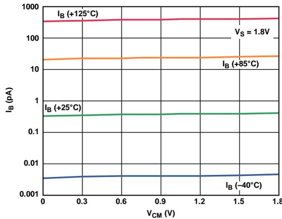
Figure 27. Input Bias Current vs. Input Common-Mode Voltage
