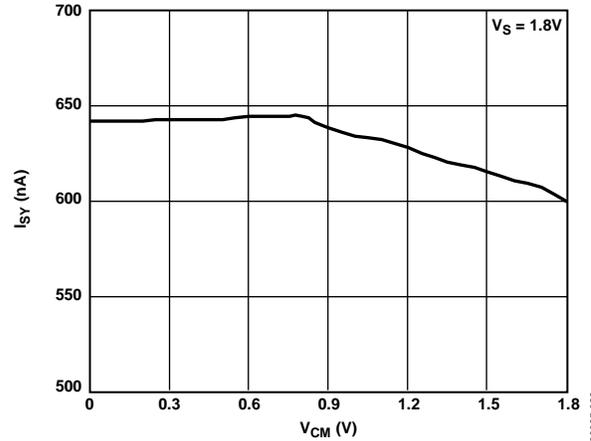
Figure 29. Supply Current vs. Input Common-Mode Voltage
