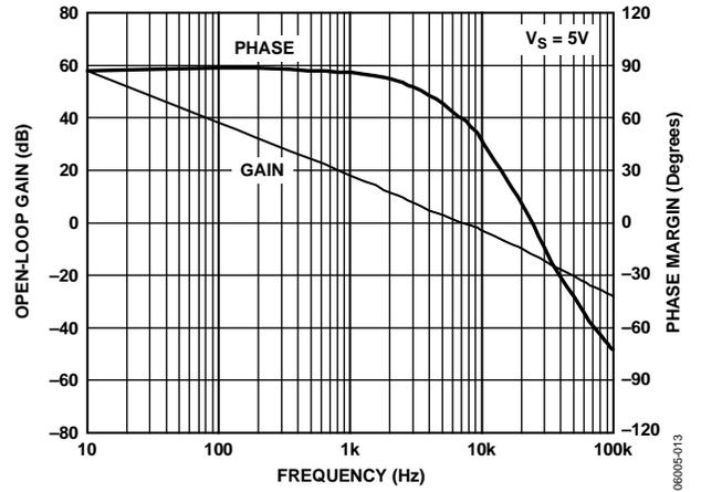
Figure 13. Open-Loop Gain and Phase vs. Frequency
