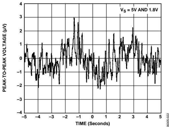
Figure 22. 0.1 Hz to 10 Hz Input Voltage Noise
