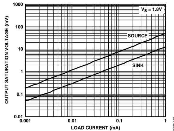
Figure 30. Output Saturation Voltage vs. Load Current
