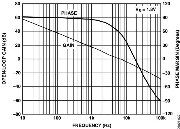
Figure 32. Open-Loop Gain and Phase vs. Frequency
