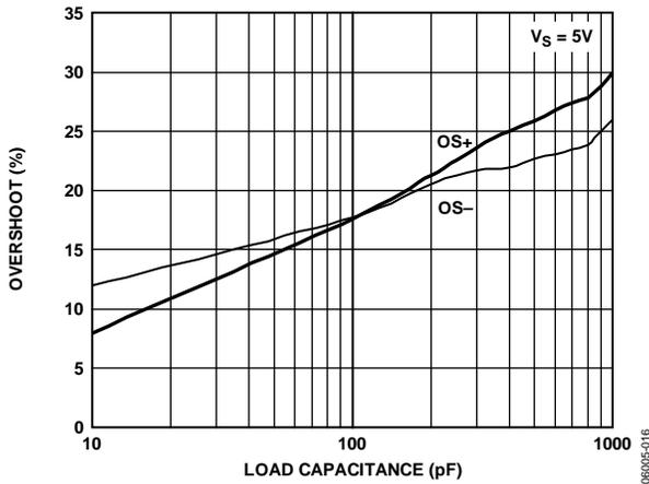
Figure 16. Small Signal Overshoot vs. Load Capacitance
