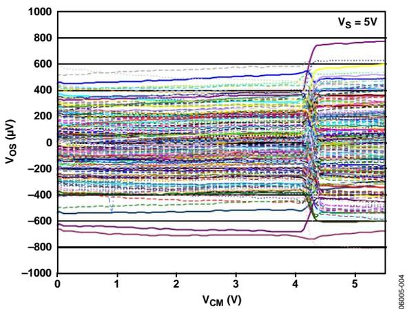
Figure 4. Input Offset Voltage vs. Common-Mode Voltage
