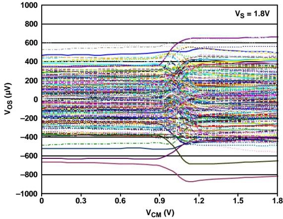
Figure 26. Input Offset Voltage vs. Input Common-Mode Voltage
