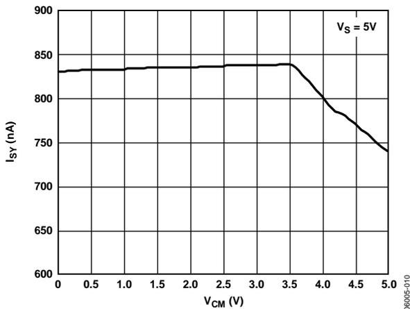
Figure 10. Supply Current vs. Input Common-Mode Voltage
