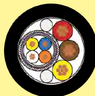
Structure Hybrid cable Data: 4x AWG26/7 Power: 3x AWG20/7
