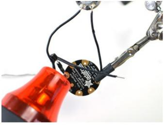
The tilt ball switch has two leads. Solder one lead to D0 on GEMMA and the other lead to GND on GEMMA.
