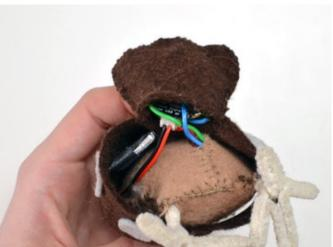
Because the GEMMA sits inside the tail of the owl, we needed to cut an additional tail piece from the brown felt included in the owl kit, then sewed it to the original tail piece to make a pocket.
