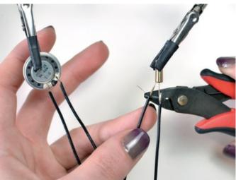
Slide a piece of the smallest diameter heat shrink tubing over each leg of the tilt ball switch to insulate the wires and solder connections.
