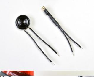
Your speaker and tilt ball switch are now ready for attaching to the rest of your circuit!
