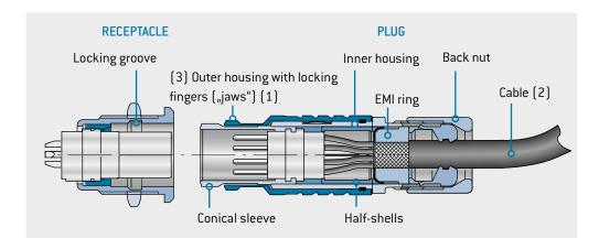
Pulling on the cable or back nut causes the locking fingers to grip harder into the locking groove in the receptacle. This prevents the connector from being disconnected.
