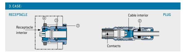
All IP 68 submersible 0DU MINI-SNAP connectors have a rated water depth of 2 m (0.2 bar) for 24 hours in accordance with IEC 60529:2013 (VDE 0470-1:2014). A watertight connector requires a sealing in a cable collet sustem.
