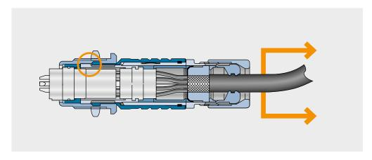
But pulling on the outer housing will cause the fingers to emerge from the locking groove, making it easy to disconnect the connector.
