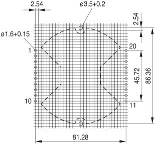
Hole arrangement view in mounting direction
