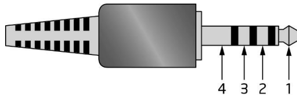
Figure 4. 4-Pin 3.5 mm (1/8 inch) Audio Jack Pin Out
