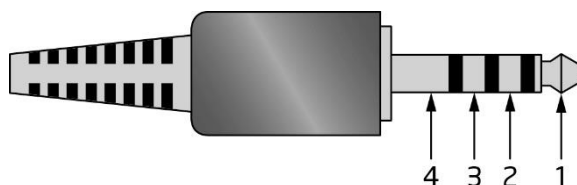
Figure 4. 4-Pin 3.5 mm (1/8 inch) Audio Jack Pin Out
