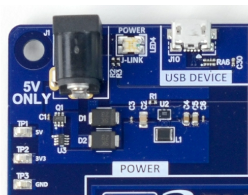
Figure 4: Power Section of Main Board
