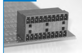
ELVA 2-Tier Aligned H/V . . . Page 23 12A / 300V
