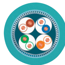
Cable cross section
