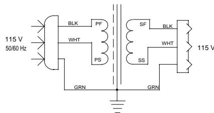
\* Leakage current between primary and secondary is typically measured at less than 10 $\mu$ A.
