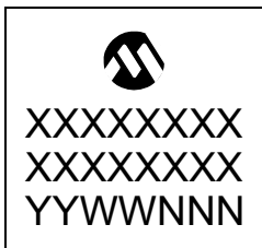
28-Lead QFN-S (6x6x0.9 mm)
