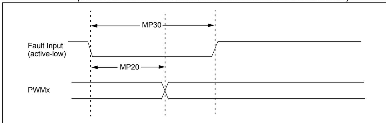
**FIGURE 30-10: HIGH-SPEED PWMx MODULE TIMING CHARACTERISTICS (dsPIC33EPXXXMC20X/50X and PIC24EPXXXMC20X DEVICES ONLY)**
