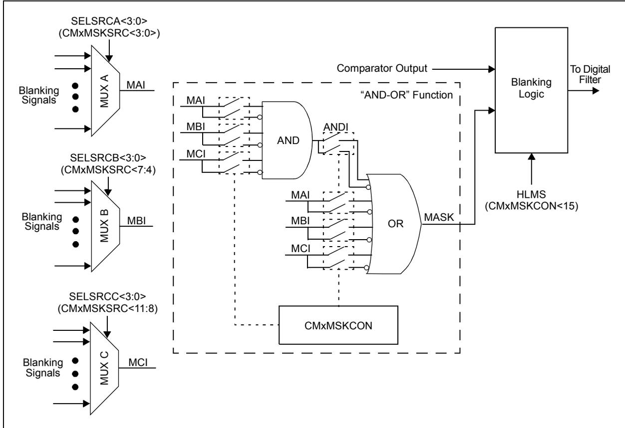
FIGURE 25-5: DIGITAL FILTER INTERCONNECT BLOCK DIAGRAM
