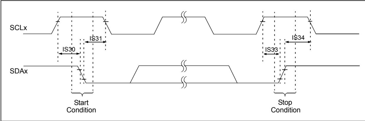
FIGURE 30-33: I2Cx BUS DATA TIMING CHARACTERISTICS (SLAVE MODE)
