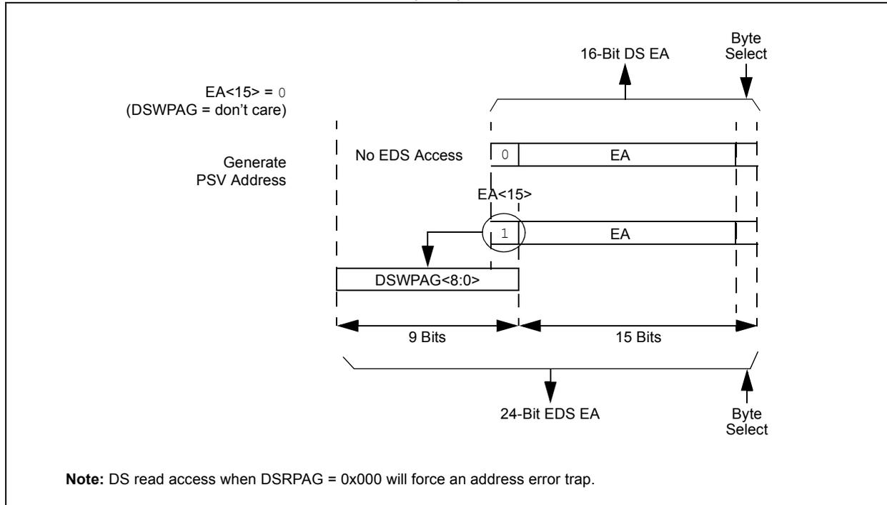
The paged memory scheme provides access to multiple 32-Kbyte windows in the EDS and PSV memory. The Data Space Page registers, DSxPAG, in combination with the upper half of Data Space address, can provide up to 16 Mbytes of additional address space in the EDS and 8 Mbytes (DSRPAG only) of PSV address space. The paged data memory space is shown in [Example 4-3](#).
