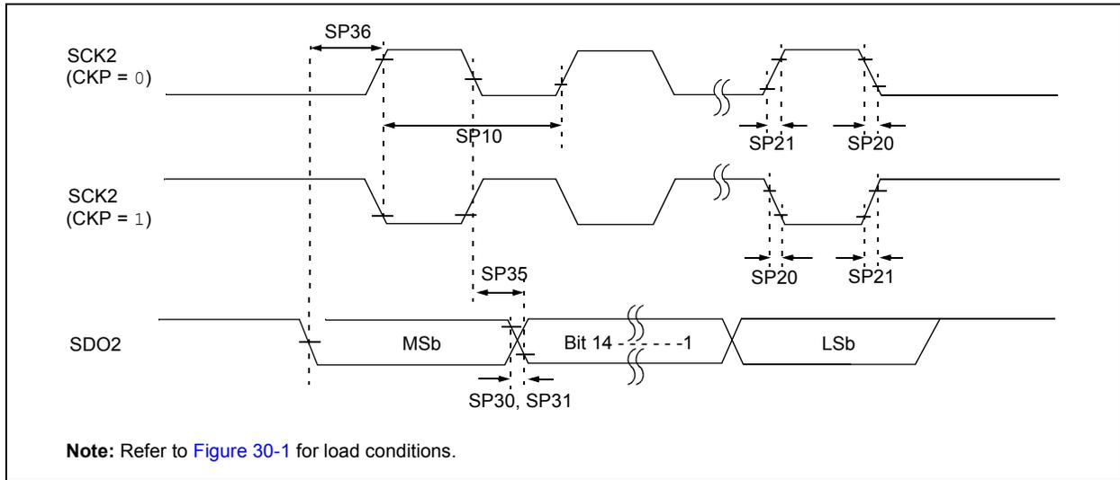
**TABLE 30-34: SPI2 MASTER MODE (HALF-DUPLEX, TRANSMIT ONLY) TIMING REQUIREMENTS**
