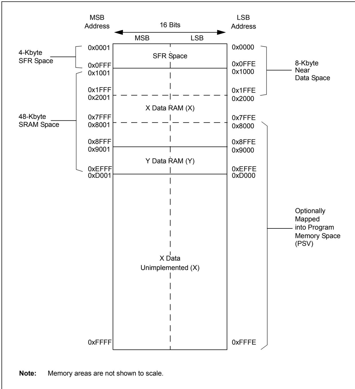
FIGURE 4-12: DATA MEMORY MAP FOR PIC24EP32GP/MC20X/50X DEVICES
