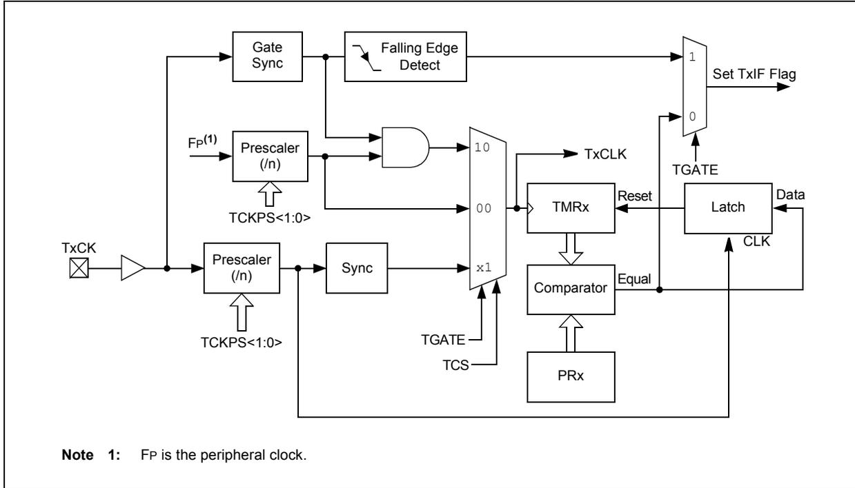
FIGURE 13-2: TYPE C TIMER BLOCK DIAGRAM (x = 3 AND 5)
