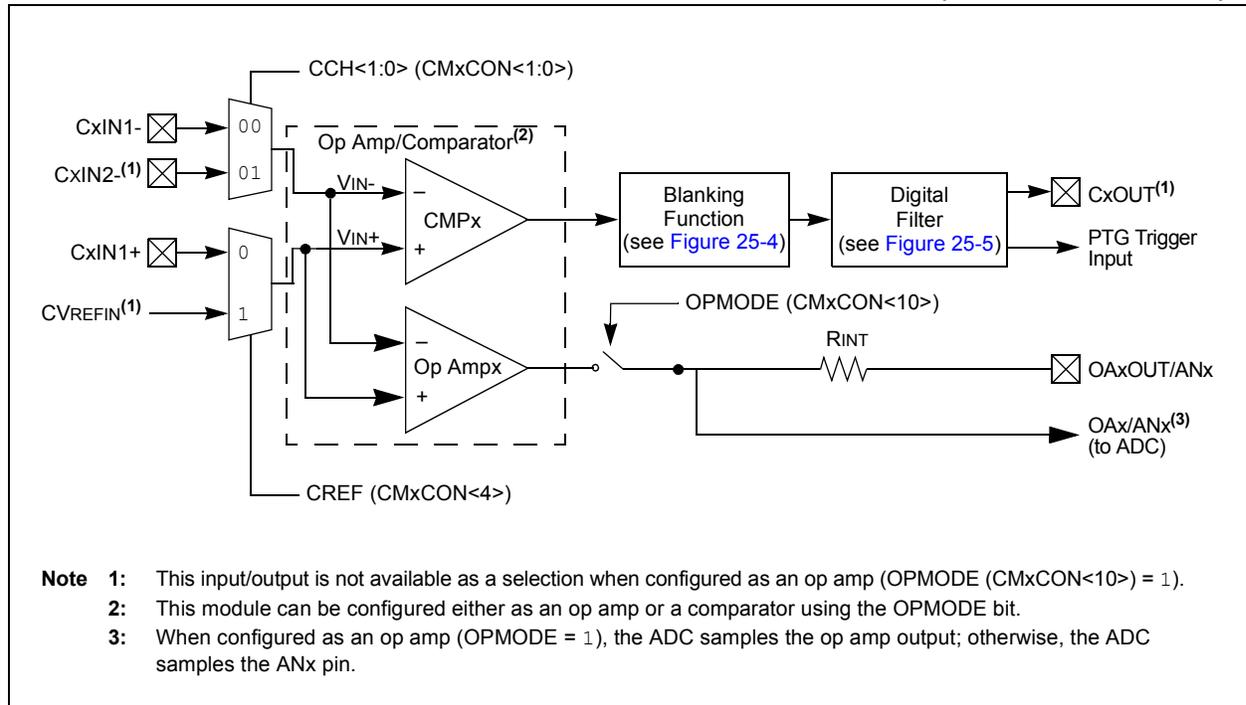
FIGURE 25-2: COMPARATOR MODULE BLOCK DIAGRAM (MODULE 4)
