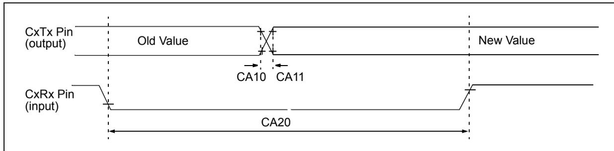
TABLE 30-51: ECANx MODULE I/O TIMING REQUIREMENTS
