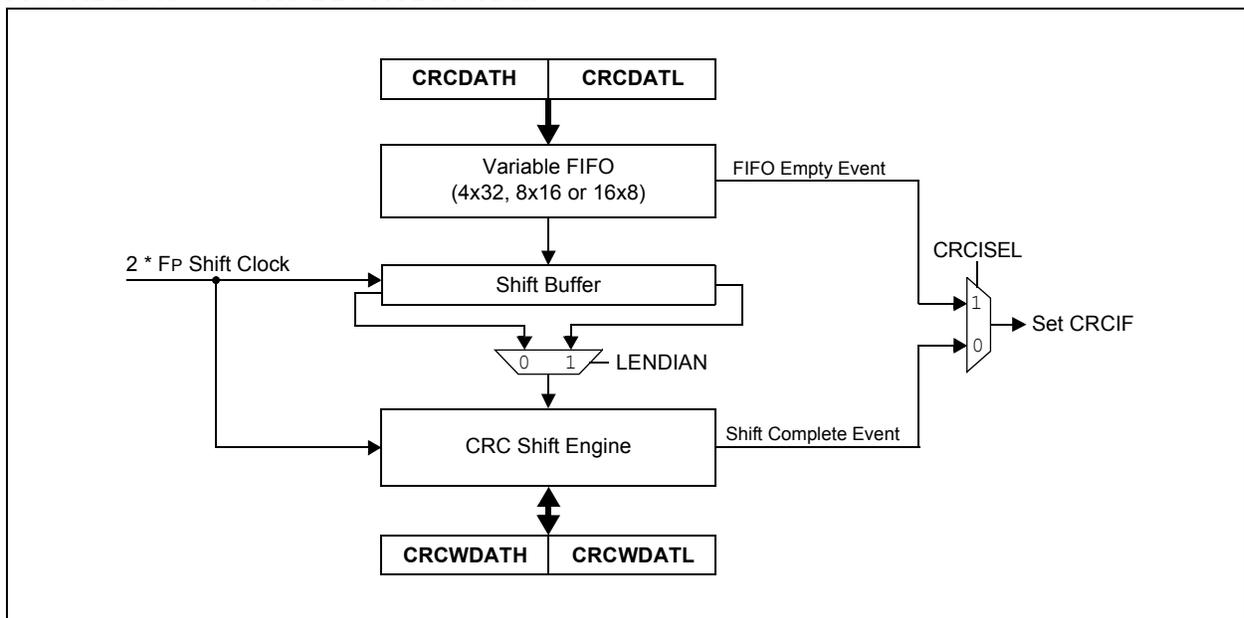
FIGURE 26-2: CRC SHIFT ENGINE DETAIL
