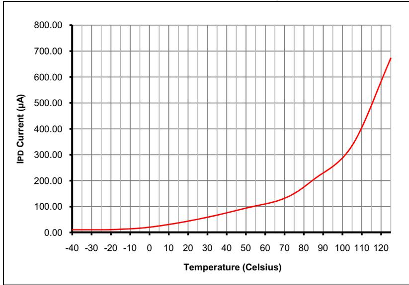
**FIGURE 32-7: TYPICAL I<sub>DOZE</sub> CURRENT @ V<sub>DD</sub> = 3.3V**
