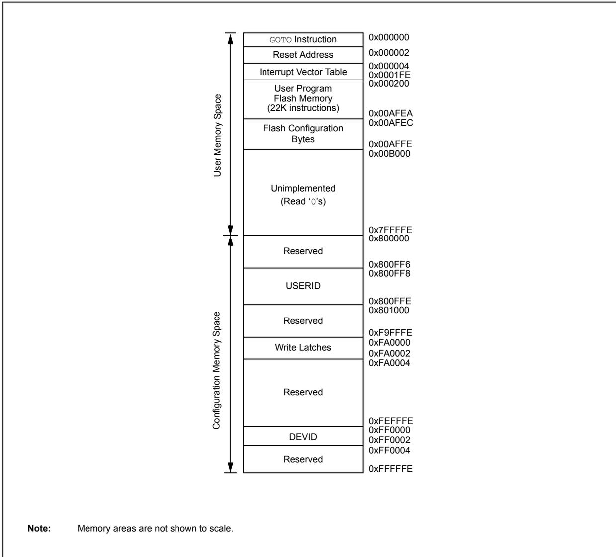
FIGURE 4-3: PROGRAM MEMORY MAP FOR dsPIC33EP128GP50X, dsPIC33EP128MC20X/50X AND PIC24EP128GP/MC20X DEVICES
