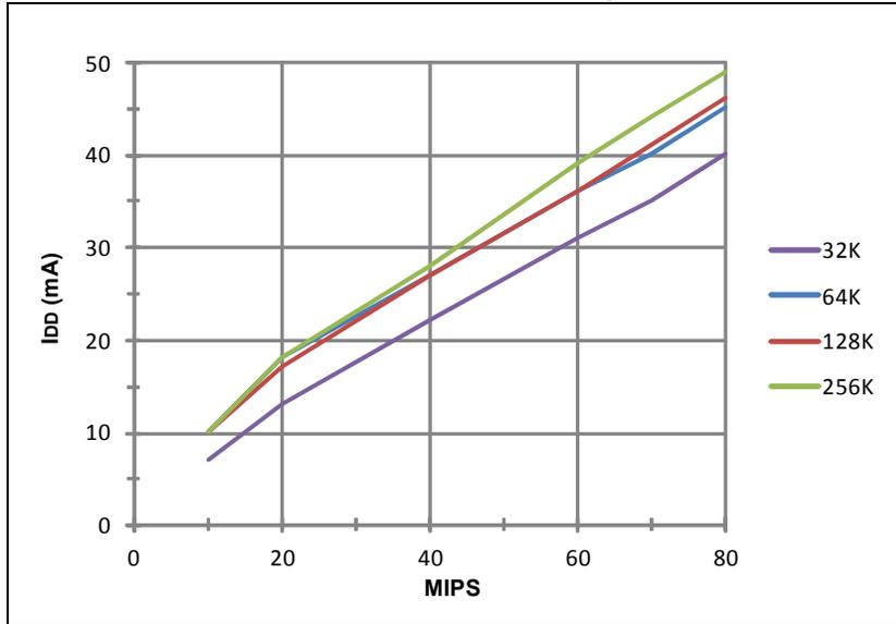
**FIGURE 32-8: TYPICAL I<sub>IDLE</sub> CURRENT @ V<sub>DD</sub> = 3.3V**
