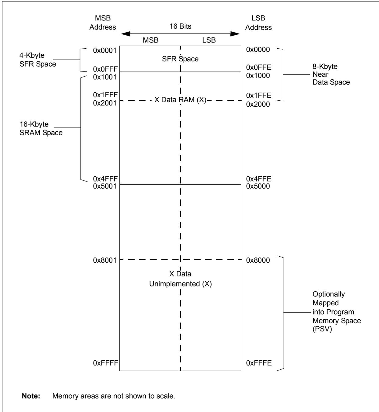
FIGURE 4-15: DATA MEMORY MAP FOR PIC24EP256GP/MC20X/50X DEVICES
