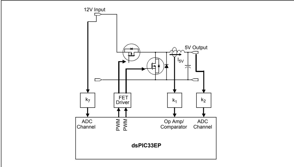
FIGURE 2-6: MULTI-PHASE SYNCHRONOUS BUCK CONVERTER
