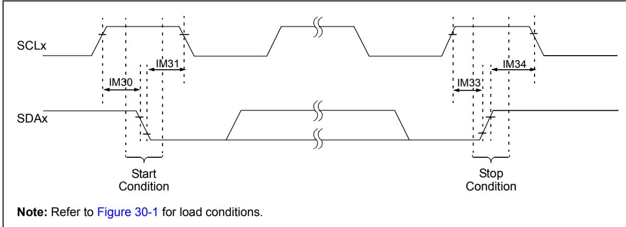
**FIGURE 30-31: I2Cx BUS DATA TIMING CHARACTERISTICS (MASTER MODE)**
