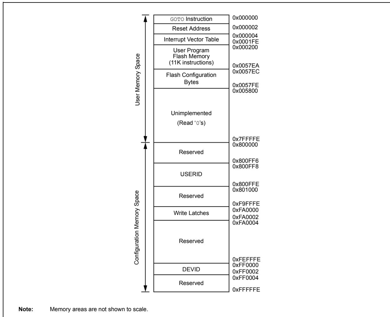
**FIGURE 4-2: PROGRAM MEMORY MAP FOR dsPIC33EP64GP50X, dsPIC33EP64MC20X/50X AND PIC24EP64GP/MC20X DEVICES**
