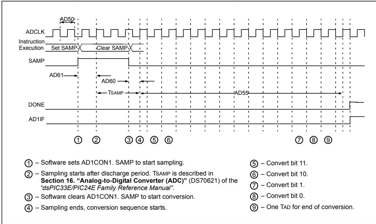
TABLE 30-60: ADC CONVERSION (12-BIT MODE) TIMING REQUIREMENTS
