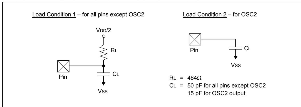
**TABLE 30-16: CAPACITIVE LOADING REQUIREMENTS ON OUTPUT PINS**
