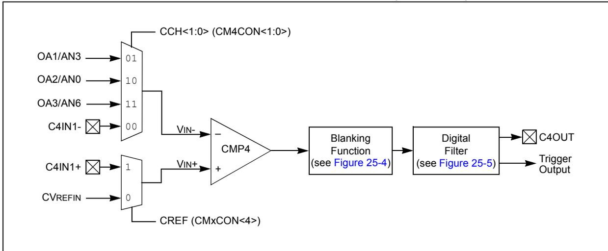
FIGURE 25-3: OP AMP/COMPARATOR VOLTAGE REFERENCE BLOCK DIAGRAM
