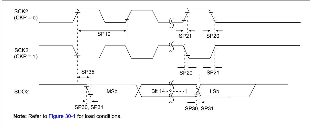
**FIGURE 30-15: SPI2 MASTER MODE (HALF-DUPLEX, TRANSMIT ONLY, CKE = 1) TIMING CHARACTERISTICS**
