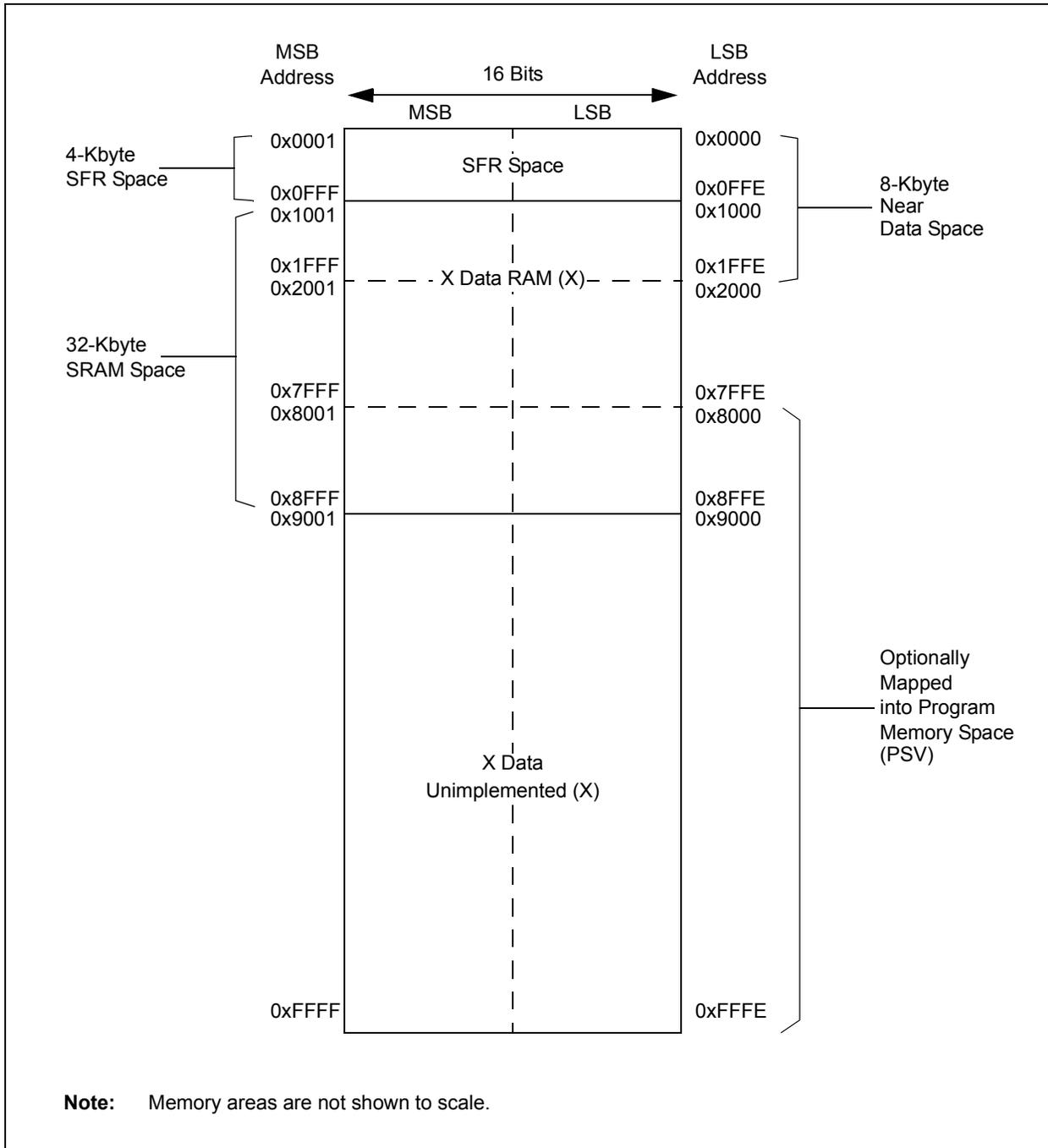
FIGURE 4-16: DATA MEMORY MAP FOR PIC24EP512GP/MC20X/50X DEVICES
