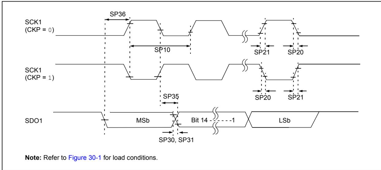
**TABLE 30-42: SPI1 MASTER MODE (HALF-DUPLEX, TRANSMIT ONLY) TIMING REQUIREMENTS**
