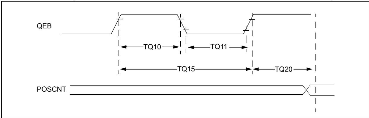
**TABLE 30-30: QEI MODULE EXTERNAL CLOCK TIMING REQUIREMENTS (dsPIC33EPXXXMC20X/50X AND PIC24EPXXXMC20X DEVICES ONLY)**
