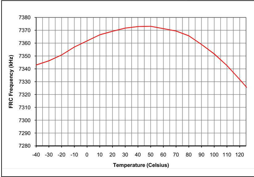
**FIGURE 32-10: TYPICAL LPRC FREQUENCY @ VDD = 3.3V**
