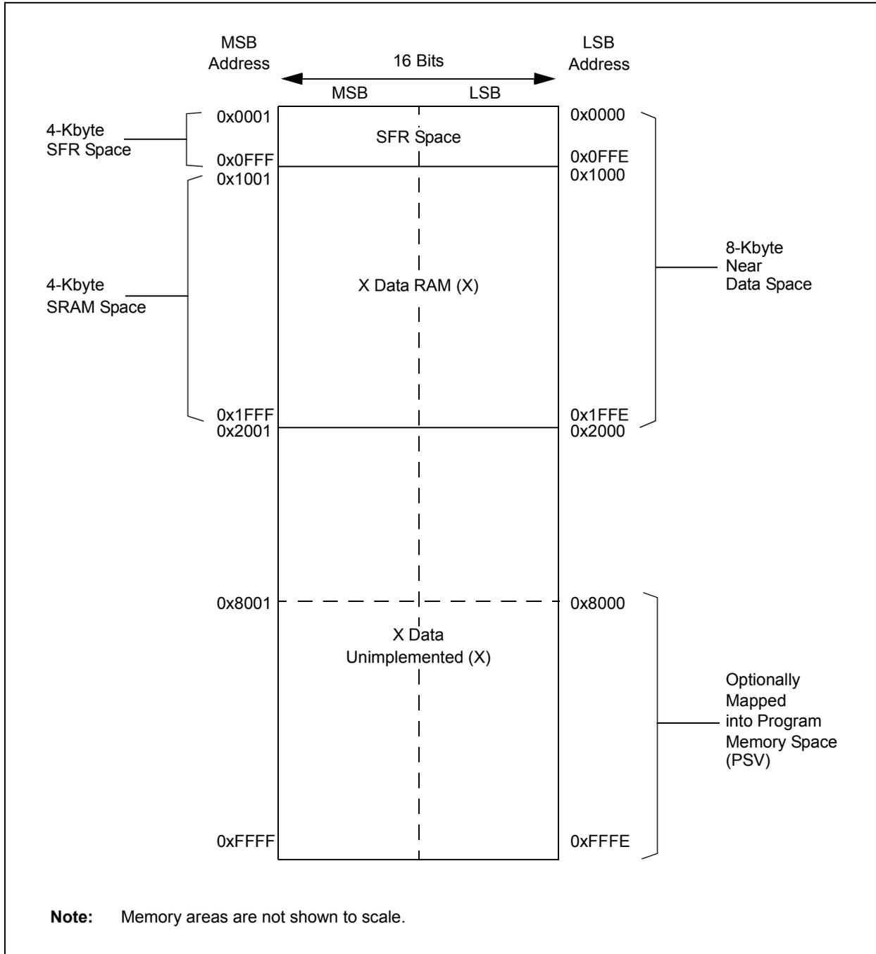
FIGURE 4-13: DATA MEMORY MAP FOR PIC24EP64GP/MC20X/50X DEVICES
