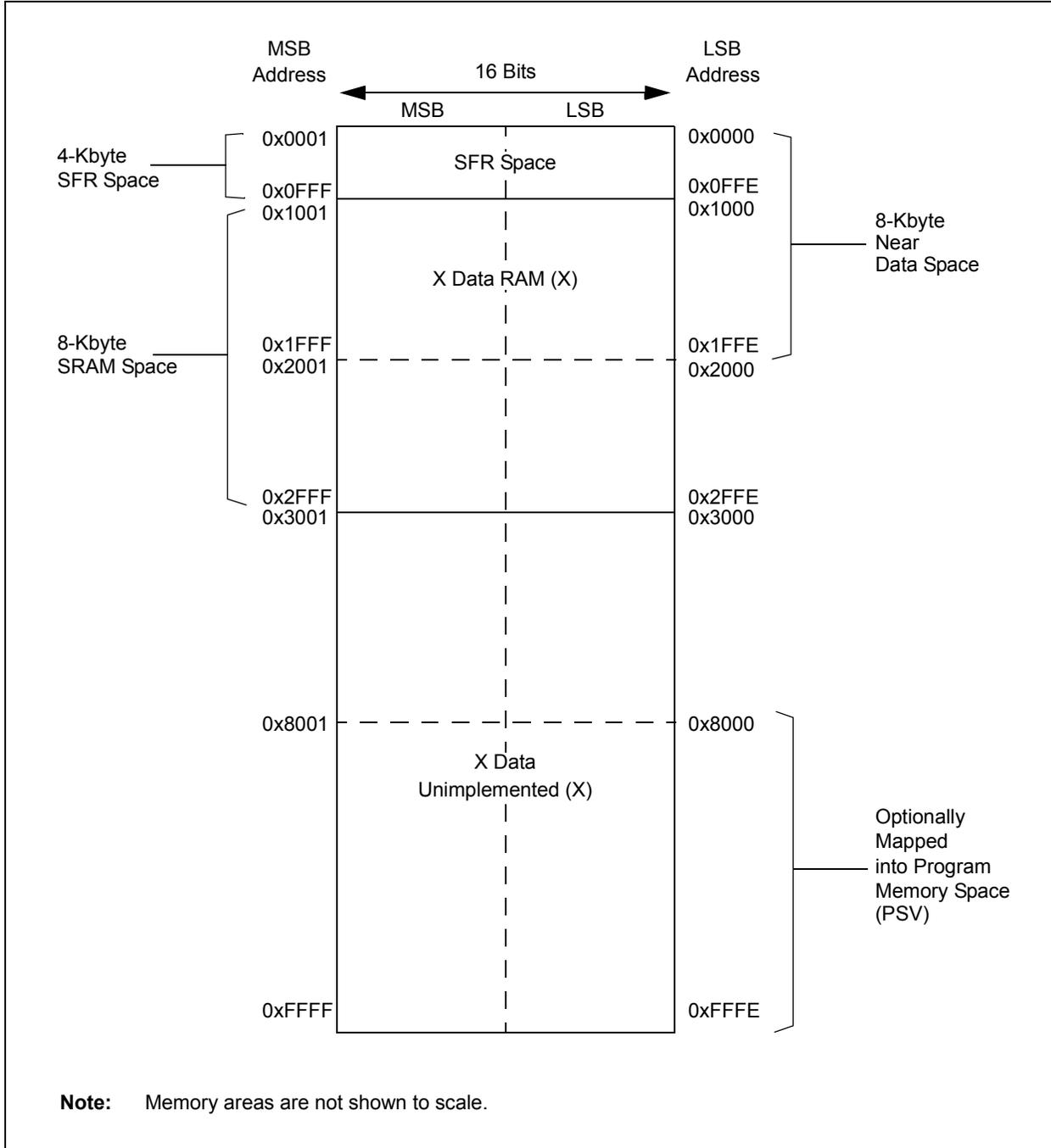
FIGURE 4-14: DATA MEMORY MAP FOR PIC24EP128GP/MC20X/50X DEVICES
