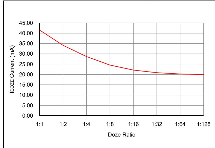
**FIGURE 32-6: TYPICAL I<sub>DD</sub> CURRENT @ V<sub>DD</sub> = 3.3V**
