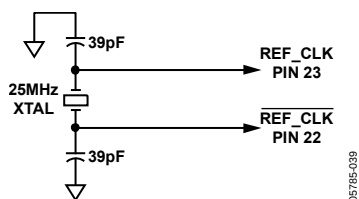
Figure 40. Crystal Configuration for Reference Clock Source
