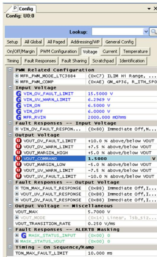
Then, click the “W” (PC to RAM) icon to write these register values to the LTC3884. After finishing this step, you will see the output voltage will change to 1.5V.
