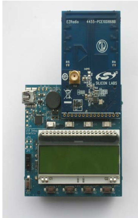
Figure 3. LCD Baseboard with Connected RF Pico Board
