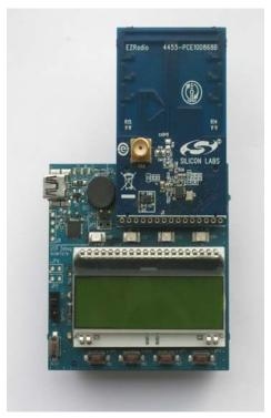
Figure 3. LCD Baseboard with Connected RF Pico Board
