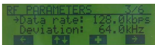
Figure 8. Menu Page: RF Parameters 3/6 (Modulation is 2GFSK)
