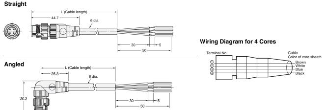
Note: The overmolding on the Standard Cable (XS5H-D42 -- 80-A) and the Oil-resistant Polyurethane Cable (XS5H-D42 -- 80-P) is black, and the overmolding of the Vibration-proof Robot Cable (XS5H-D42□-□81-F) is gray
