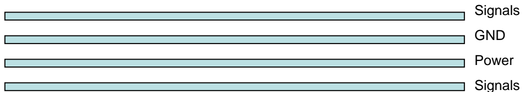
Figure 21: Typical 4-layer PCB construction
