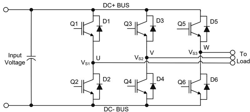
**Figure 4** Three phase inverter
