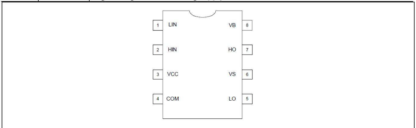
Figure 3 2ED2304S06F lead assignments PG-DSO-8 (top view)
