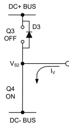
Figure 8 Q4 conducting
