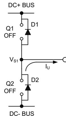
Figure 6 D2 conducting
