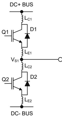
Figure 9 Parasitic Elements
