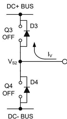
Figure 7 D3 conducting
