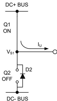
Figure 5 Q1 conducting
