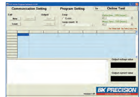
Pass/Fail test monitors maximum and minimum voltage and current values over a specified period of time.
