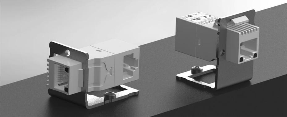
With the universal Keystone Mounting Bracket Z-5-KMB, Network Isolators featuring Keystone interfaces (as well as all other Keystone-compatible modules) can be easily and securely mounted to surfaces. The brackets can be assembled for either an upright (0°), or a rotated (90°) position, and the symmetrical cut-out allows for upside-down (180°) and rotated (270°) positions, providing four possible module mounting options.
