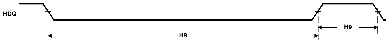
Figure 5-39. HDQ/1-Wire Break (Reset) Timing
