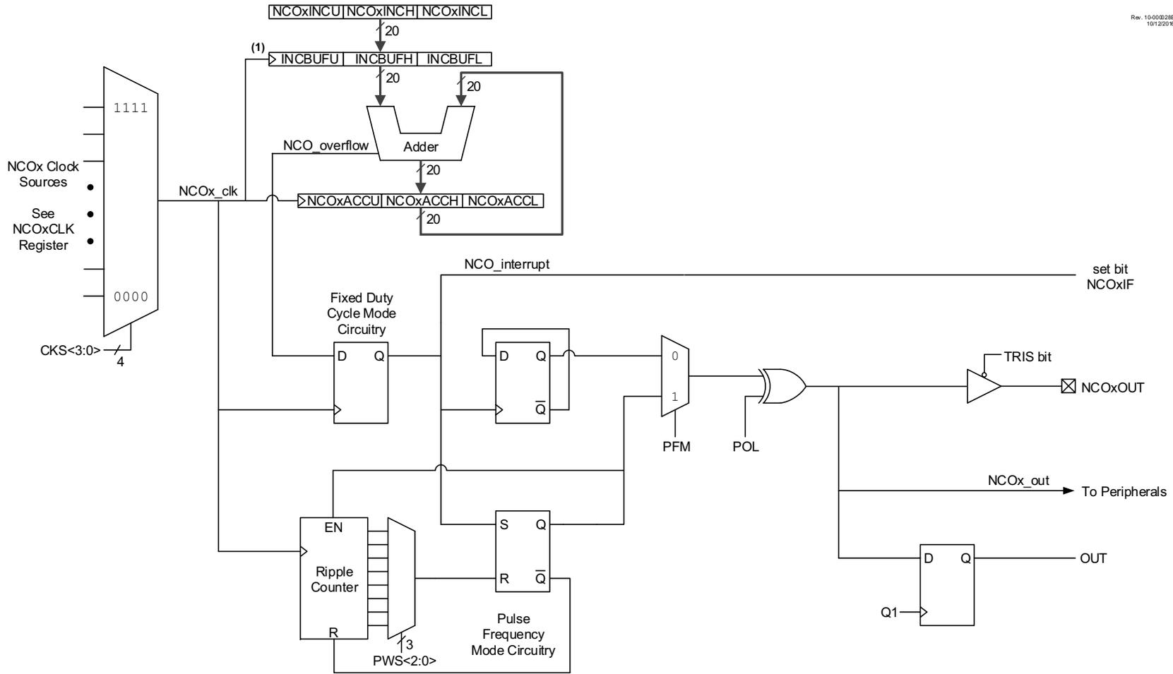
**Note 1:** The increment registers are double-buffered to allow for value changes to be made without first disabling the NCO module. The full increment value is loaded into the buffer registers on the second rising edge of the NCOx\_clk signal that occurs immediately after a write to NCOxINCL register. The buffers are not user-accessible and are shown here for reference.
