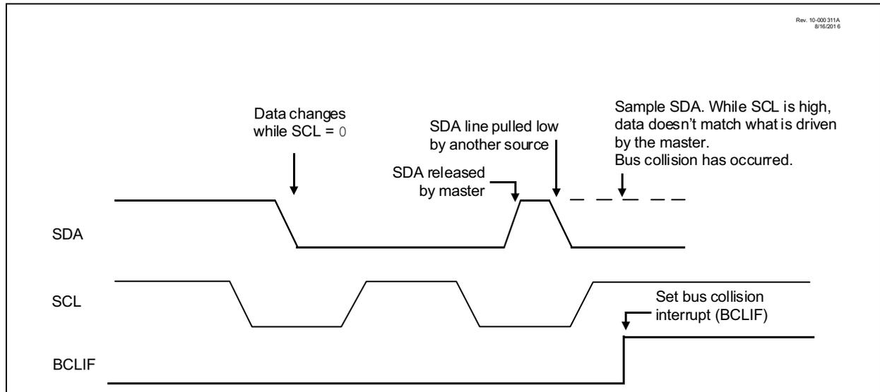
If transmission was in progress when the bus collision occurred, the SDA and SCL lines are released. If a Repeated Start, Stop or Acknowledge was in progress when the bus collision occurred, the action is aborted; the SDA and SCL lines are released. The BCLIF condition must be cleared by software to allow an ACK to be shifted out on the bus again, until then the module will always respond with a NACK. Refer to [Figure 33-24](#) for a detailed timing diagram of a transaction in Multi-Master mode.
