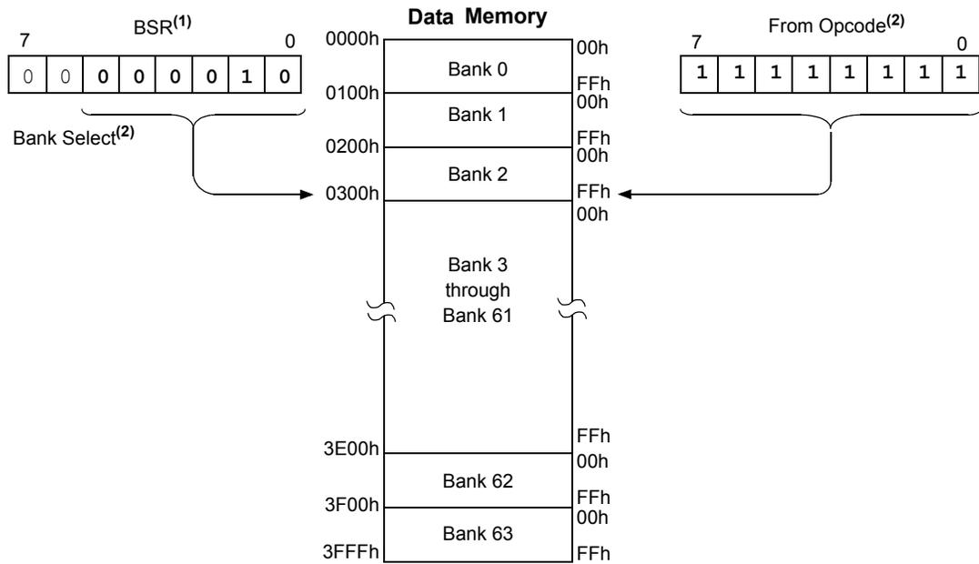
**Note 1:** The Access RAM bit of the instruction can be used to force an override of the selected bank (BSR<5:0>) to the registers of the Access Bank.
