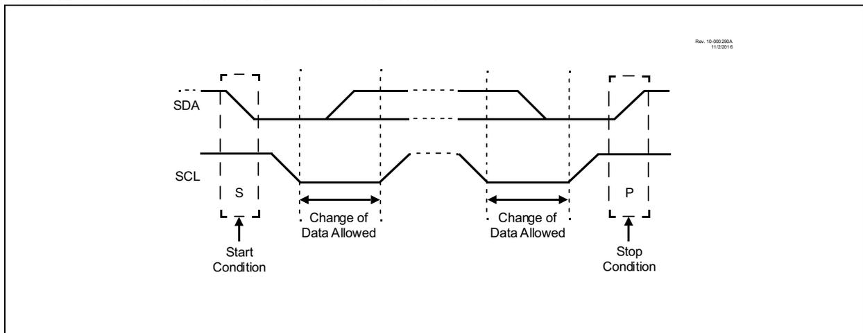
**Note:** At least one SCL low time must appear before a Stop is valid. Therefore if the SDA line goes low then high again while the SCL line is high, only the Start condition is detected.
