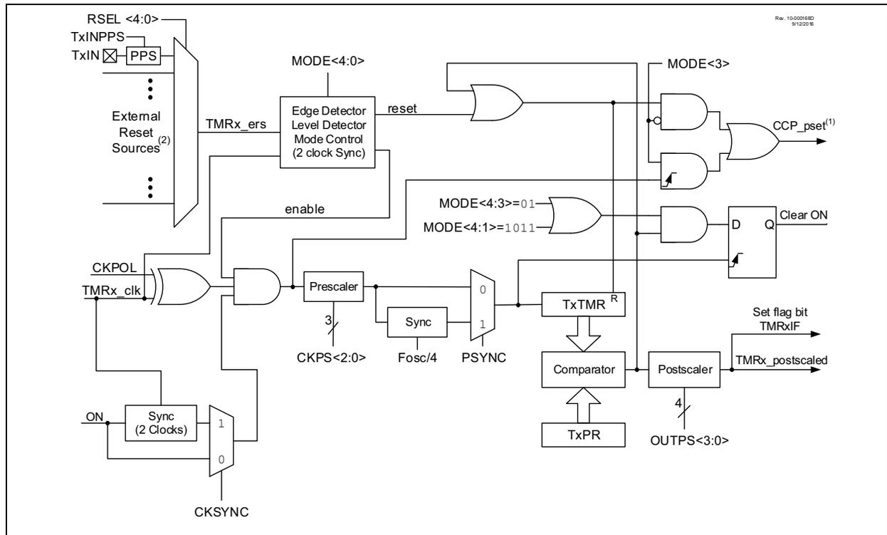
**FIGURE 22-2: TIMER2 CLOCK SOURCE BLOCK DIAGRAM**
