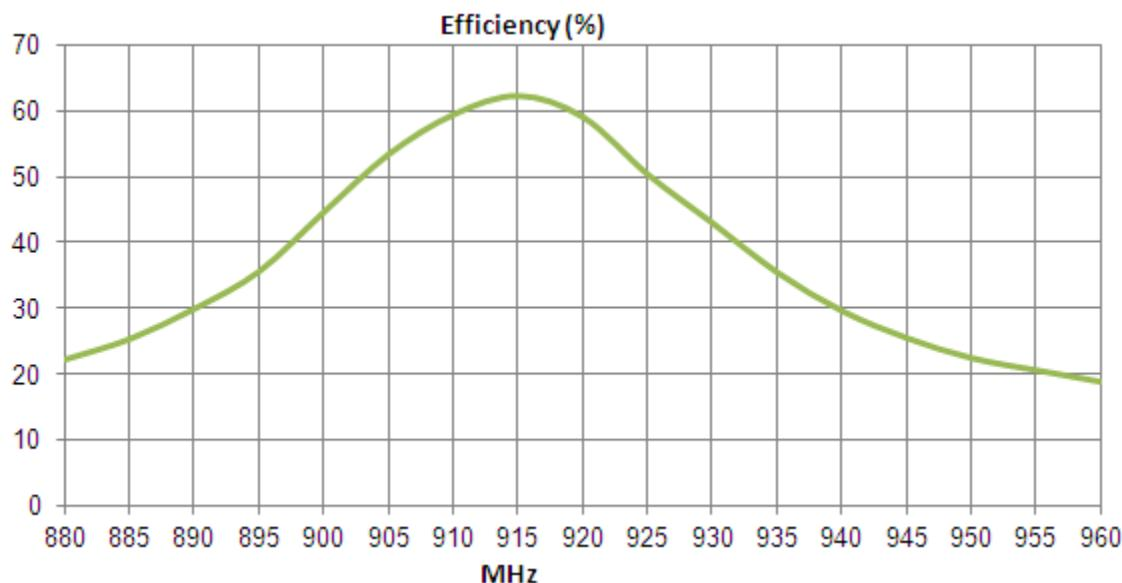
Figure 4. Efficiency of 915 MHz ISM Band Antenna ILA.01
