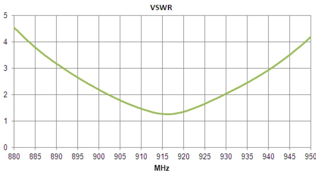
**Figure 3.** VSWR of 915 MHz ISM Band Antenna ILA.01
