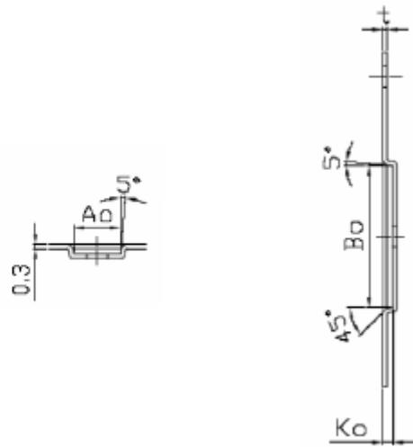
**Figure 13.** Tape dimensions for the ILA.01.
