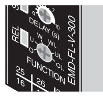
When supply voltage U is applied, output relay "R" picks up (yellow "REL" LED is ON) and the starting override (START) starts (green "U" LED flashes). During the starting override, modifications to the measured value have no influence on the position of the output relay. Once the starting override has elapsed, the green "U" LED lights up permanently. For all functions the "MIN" and "MAX" LEDs flash alternately if the minimum value selected is greater than the maximum value.
