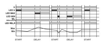
If the error memory has been activated (WIN + LATCH) and the measured voltage has fallen below the value set at the "MIN" controller for longer than the set response delay, output relay "R" does not pick up if the minimum value is exceeded. If the measured voltage has exceeded the value set at the "MAX" controller for longer than the set response delay, output relay "R" likewise does not pick up when the voltage falls below the maximum value.
