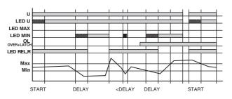
If the measured voltage falls below the value set at the "MIN" controller, the set response delay (DELAY) starts (red "MIN" LED flashes). After the delay time has elapsed (red "MIN" LED is ON), output relay "R" drops out (yellow "REL" LED is OFF). If the measured voltage exceeds the value set at the "MAX" controller, output relay "R" picks up again (yellow "REL" LED is ON).
