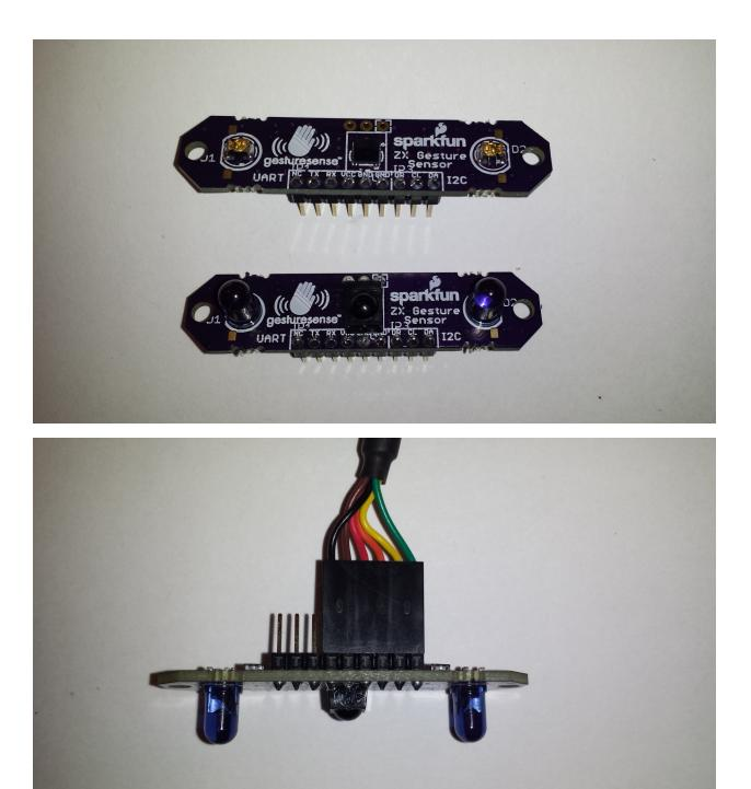
The ZX/SP sensor has labeled connections with UART and I2C separated. This makes it easy to connect ready-made connectors (like the FTDI UART connector) directly to the ZX sensor pins (as shown). Similarly, the I2C connection pins may connect to any two-wire interface using the ZX sensor as the I2C slave, and any embedded or external processor as the I2C master.
