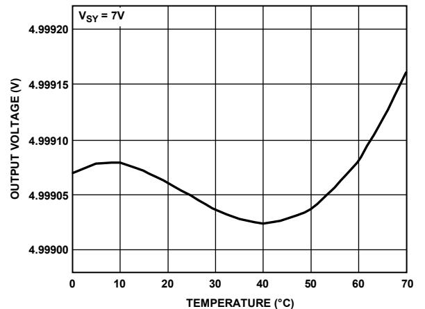
Figure 83. ADR4550 C Grade Output Voltage vs. Temperature
