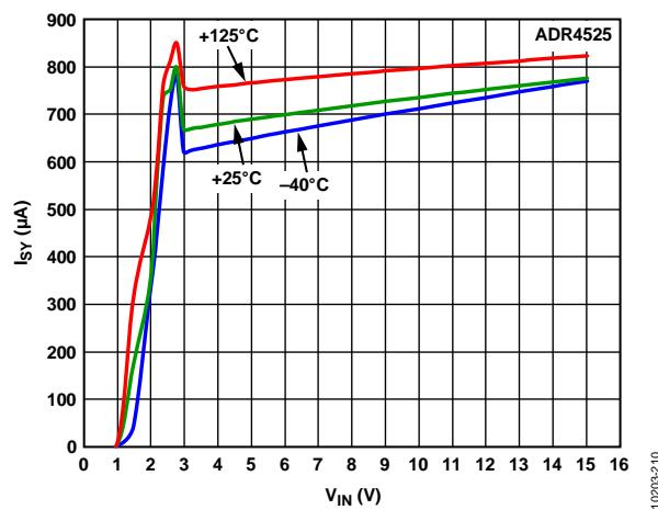
Figure 23. ADR4525 Supply Current vs. Supply Voltage
