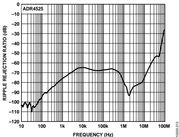
Figure 26. ADR4525 Ripple Rejection Ratio vs. Frequency
