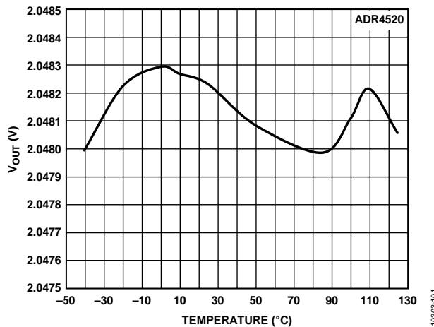
Figure 3. ADR4520 B Grade Output Voltage vs. Temperature
