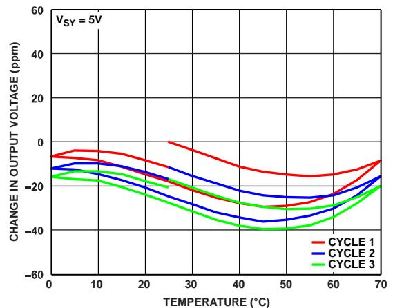
Figure 91. Change in Output Voltage over Three Full Temperature Cycles ( $0^{\circ}\text{C}$  to  $70^{\circ}\text{C}$ )
