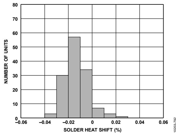
Figure 82. ADR4550 Solder Heat Resistance Shift (3 x Reflow)
