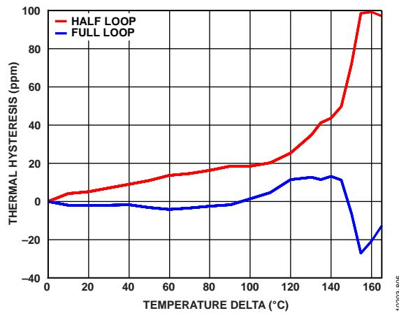
Figure 93. Thermal Hysteresis for Increasing Temperature Range
