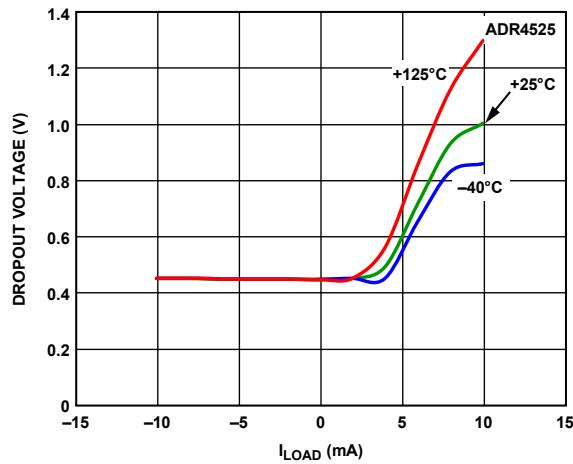
Figure 19. ADR4525 Dropout Voltage vs. Load Current
