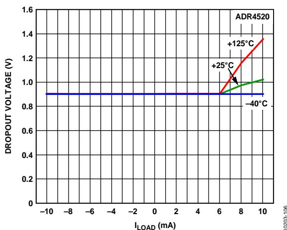
Figure 5. ADR4520 Dropout Voltage vs. Load Current
