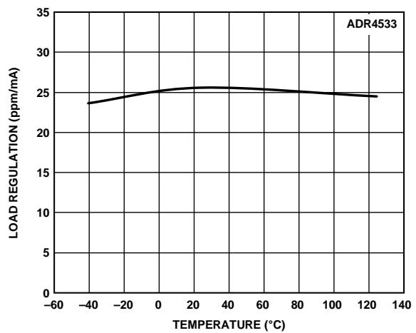
Figure 46. ADR4533 Load Regulation vs. Temperature (Sourcing)
