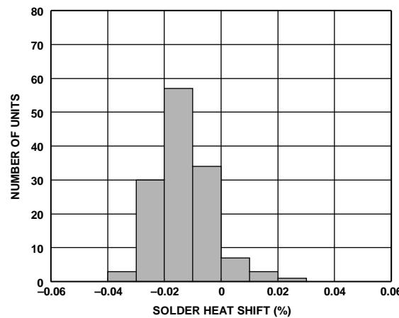
Figure 55. ADR4533 Solder Heat Resistance Shift (3 x Reflow)
