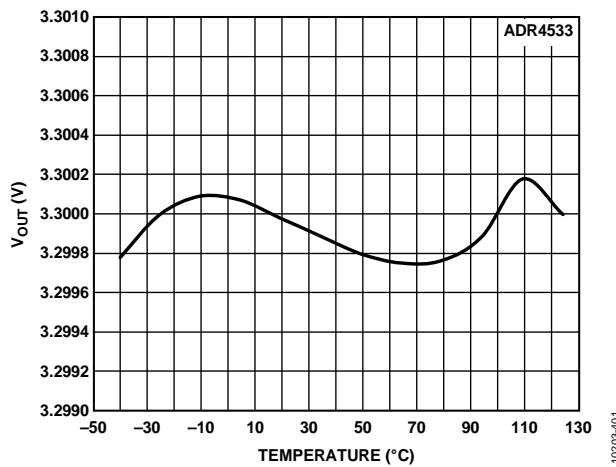
Figure 43. ADR4533 B Grade Output Voltage vs. Temperature
