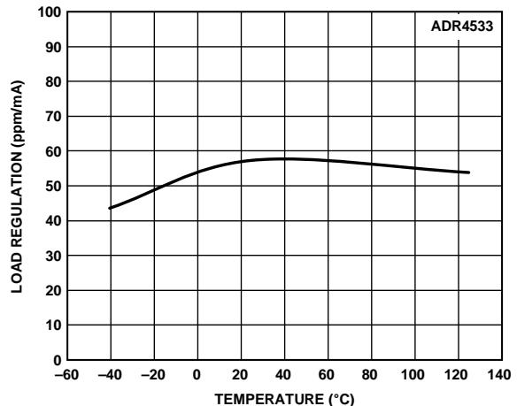
Figure 47. ADR4533 Load Regulation vs. Temperature (Sinking)
