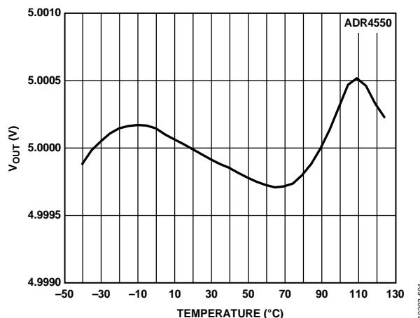
Figure 70. ADR4550 B Grade Output Voltage vs. Temperature
