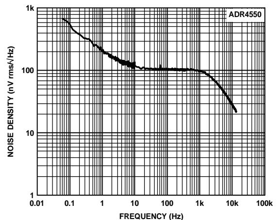
Figure 78. ADR4550 Output Noise Spectral Density
