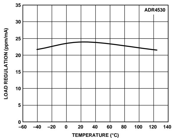
Figure 33. ADR4530 Load Regulation vs. Temperature (Sourcing)
