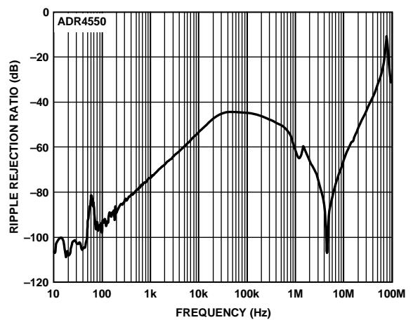
Figure 79. ADR4550 Ripple Rejection Ratio vs. Frequency
