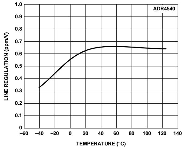
Figure 61. ADR4540 Line Regulation vs. Temperature
