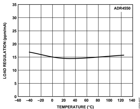
Figure 73. ADR4550 Load Regulation vs. Temperature (Sourcing)
