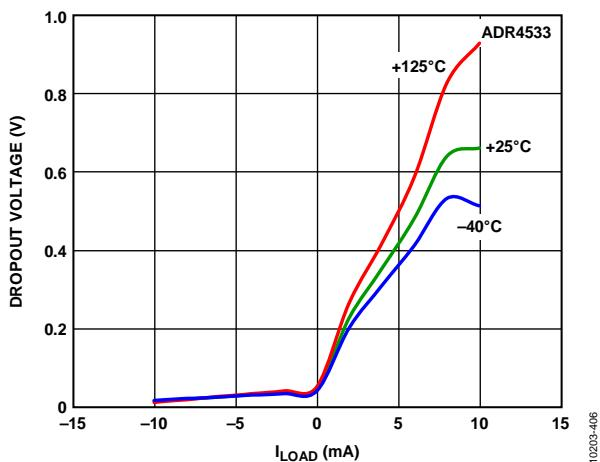
Figure 45. ADR4533 Dropout Voltage vs. Load Current
