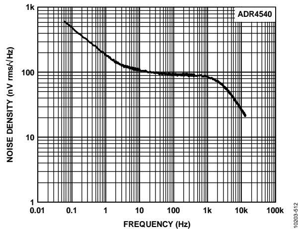
Figure 64. ADR4540 Output Noise Spectral Density
