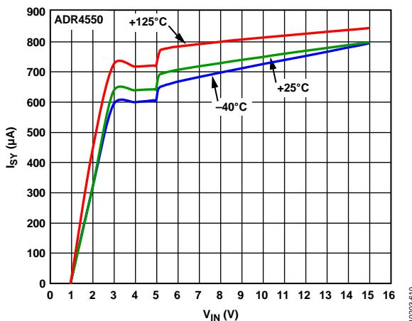
Figure 76. ADR4550 Supply Current vs. Supply Voltage
