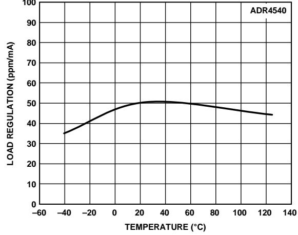
Figure 60. ADR4540 Load Regulation vs. Temperature (Sinking)
