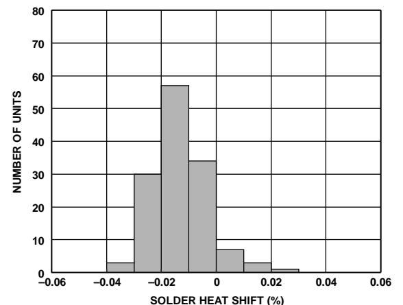
Figure 15. ADR4520 Solder Heat Resistance Shift (3 × Reflow)
