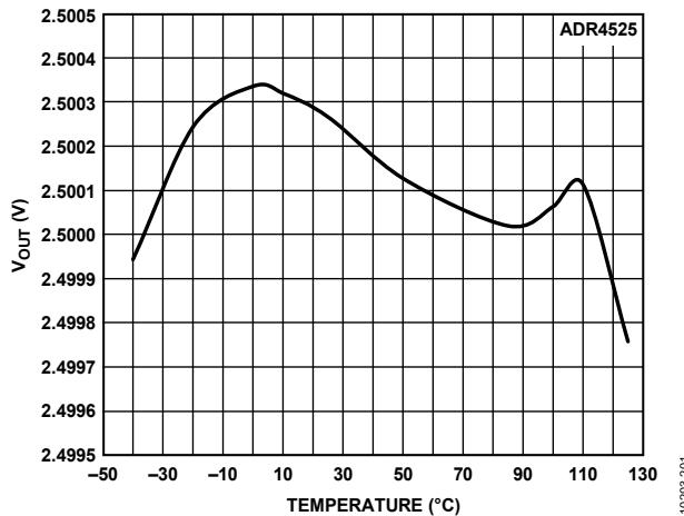
Figure 16. ADR4525 B Grade Output Voltage vs. Temperature
