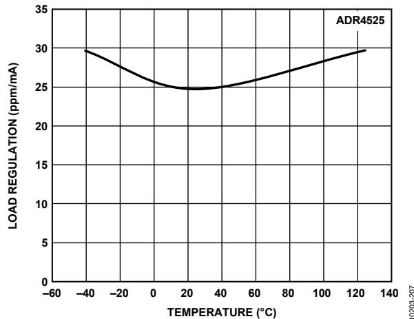
Figure 20. ADR4525 Load Regulation vs. Temperature (Sourcing)
