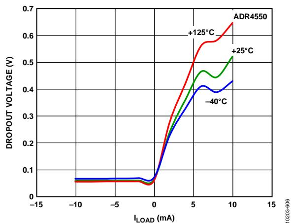
Figure 72. ADR4550 Dropout Voltage vs. Load Current
