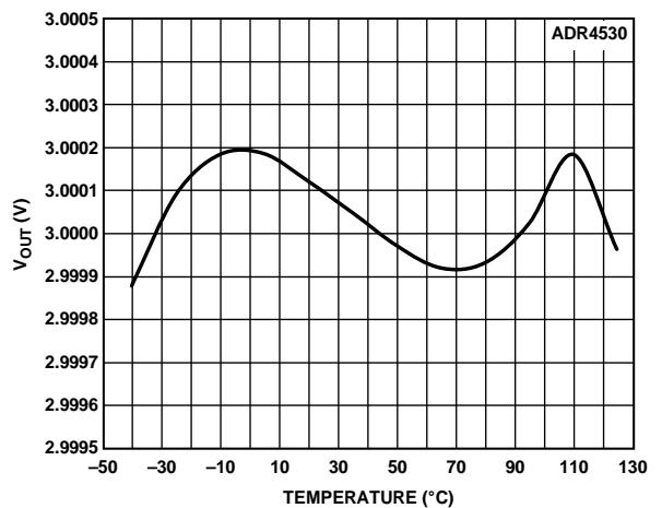
Figure 30. ADR4530 B Grade Output Voltage vs. Temperature
