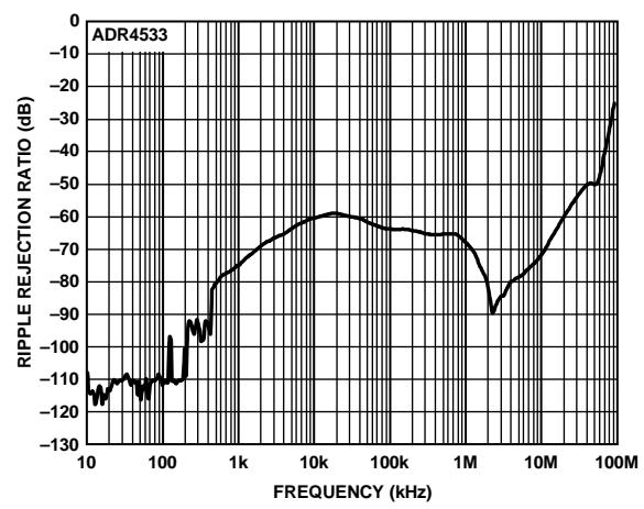
Figure 52. ADR4533 Ripple Rejection Ratio vs. Frequency
