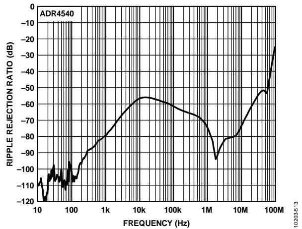
Figure 65. ADR4540 Ripple Rejection Ratio vs. Frequency
