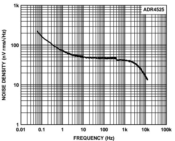
Figure 25. ADR4525 Output Noise Spectral Density
