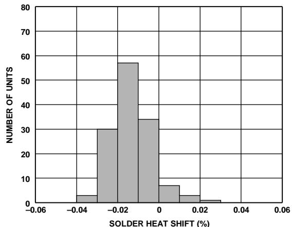
Figure 42. ADR4530 Solder Heat Resistance Shift (3 × Reflow)
