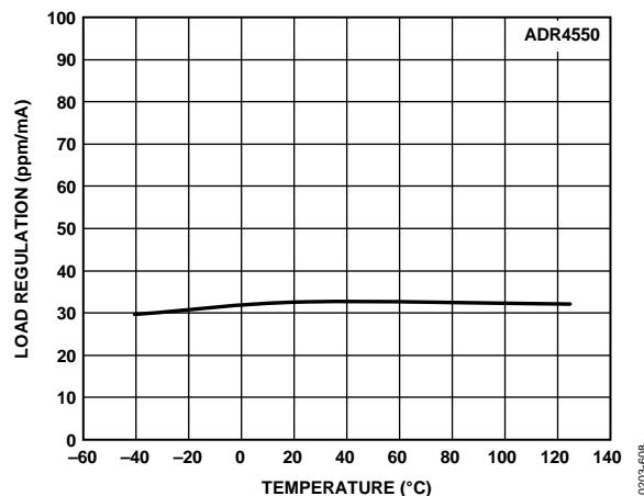
Figure 74. ADR4550 Load Regulation vs. Temperature (Sinking)
