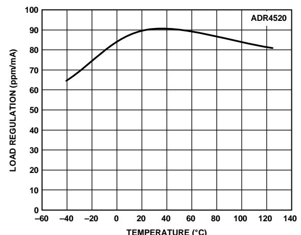
Figure 7. ADR4520 Load Regulation vs. Temperature (Sinking)
