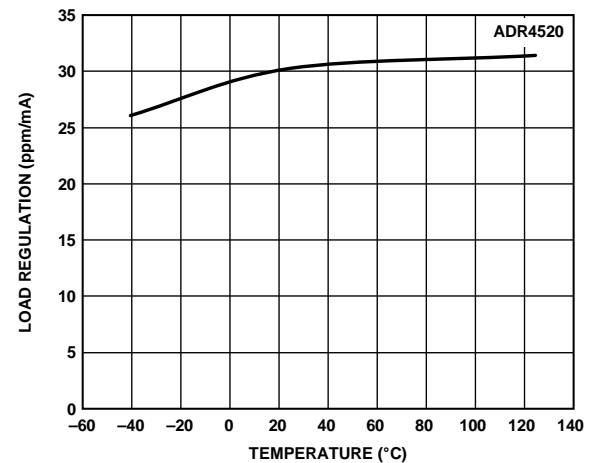
Figure 6. ADR4520 Load Regulation vs. Temperature (Sourcing)
