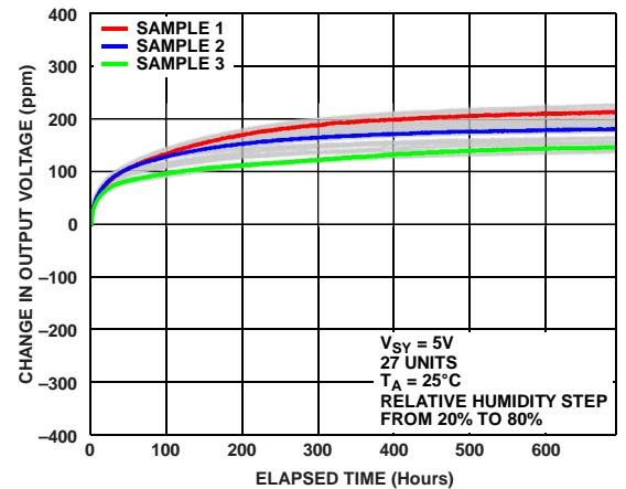
Figure 94. Change in Output Voltage vs. Time After Humidity Step Change (20% to 80% Relative Humidity)
