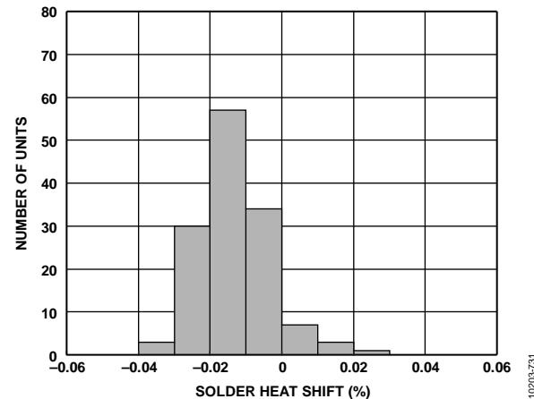
Figure 29. ADR4525 Solder Heat Resistance Shift (3 × Reflow)
