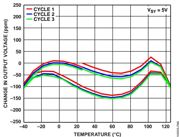
Figure 89. Change in Output Voltage over Three Full Temperature Cycles ( $-40^{\circ}\text{C}$  to  $+125^{\circ}\text{C}$ )
