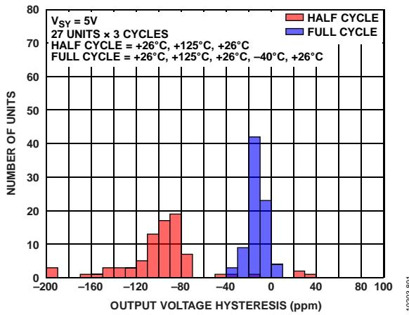
Figure 90. Histogram Showing the Temperature Hysteresis of the Output Voltage ( $-40^{\circ}\text{C}$  to  $+125^{\circ}\text{C}$ )
