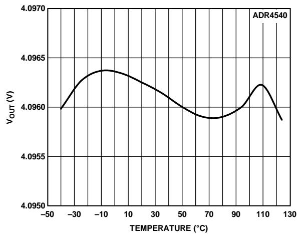
Figure 56. ADR4540 B Grade Output Voltage vs. Temperature
