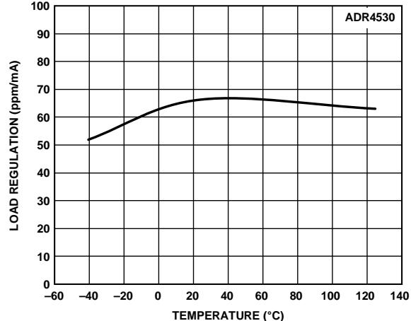
Figure 34. ADR4530 Load Regulation vs. Temperature (Sinking)
