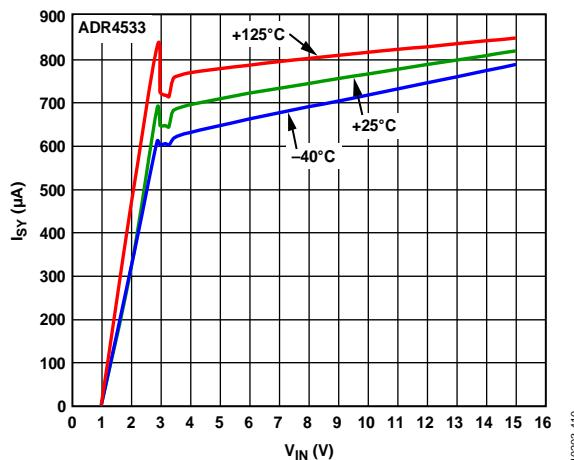
Figure 49. ADR4533 Supply Current vs. Supply Voltage
