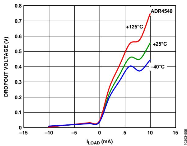
Figure 58. ADR4540 Dropout Voltage vs. Load Current
