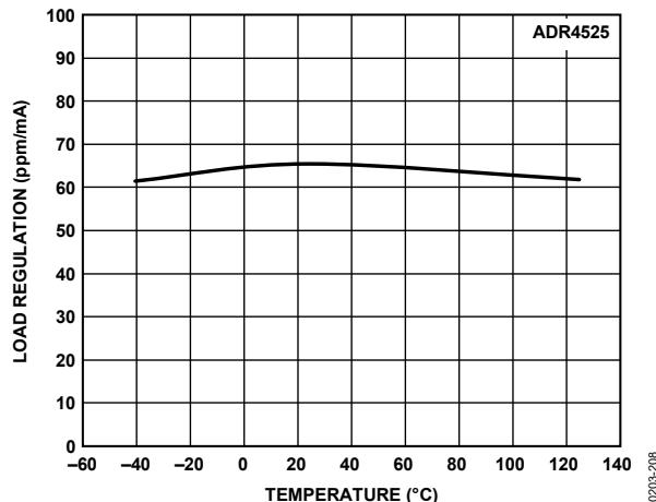
Figure 21. ADR4525 Load Regulation vs. Temperature (Sinking)
