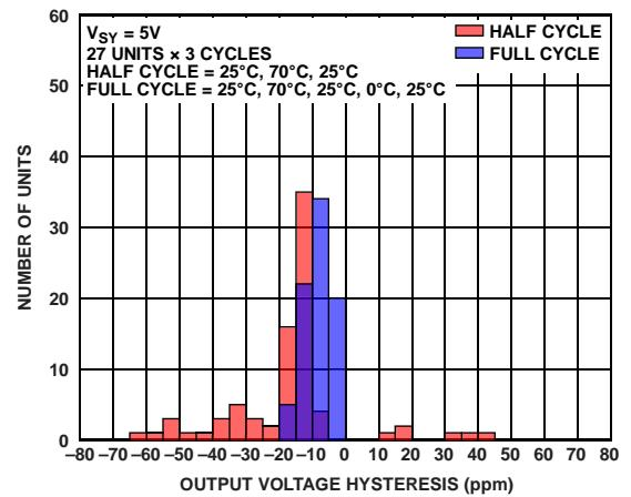
Figure 92. Histogram Showing the Temperature Hysteresis of the Output Voltage ( $0^{\circ}\text{C}$  to  $70^{\circ}\text{C}$ )
