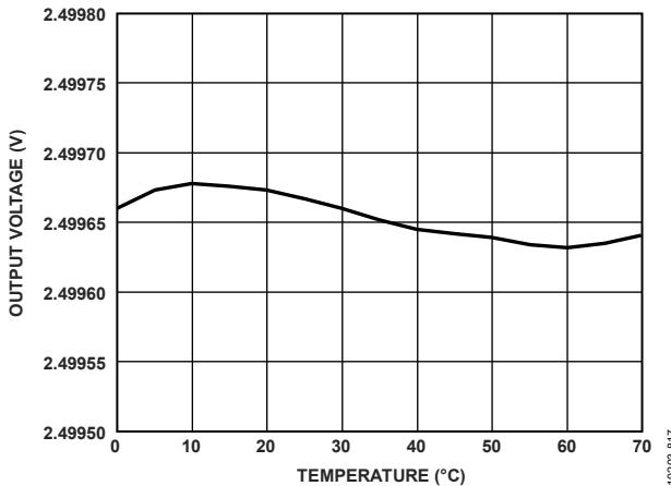
Figure 17. ADR4525 C Grade Output Voltage vs. Temperature
