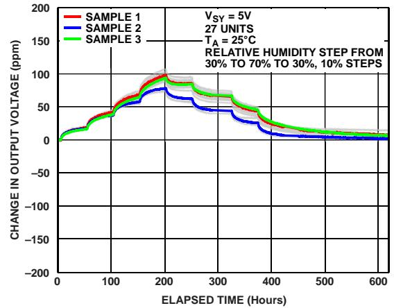
Figure 95. Change in Output Voltage vs. Time for 10% Humidity Steps (30% to 70% to 30% Relative Humidity in 10% Steps)
