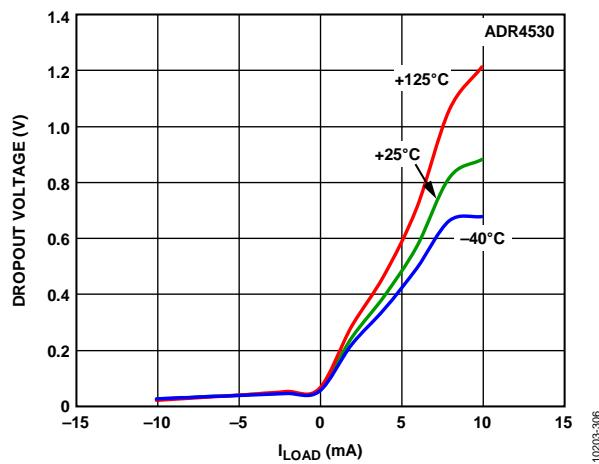
Figure 32. ADR4530 Dropout Voltage vs. Load Current
