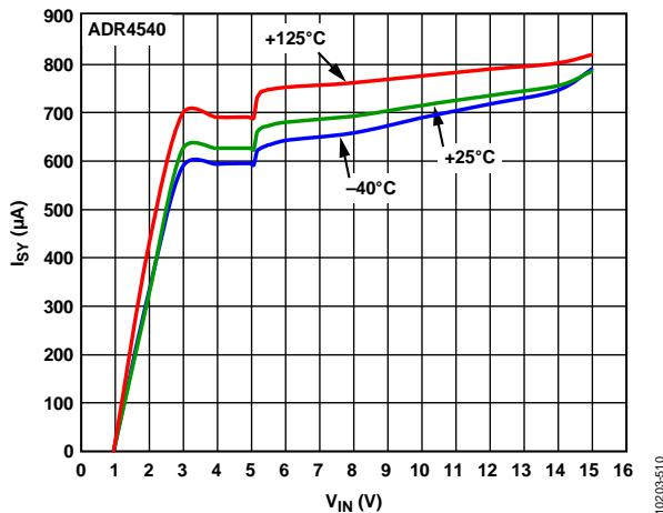
Figure 62. ADR4540 Supply Current vs. Supply Voltage
