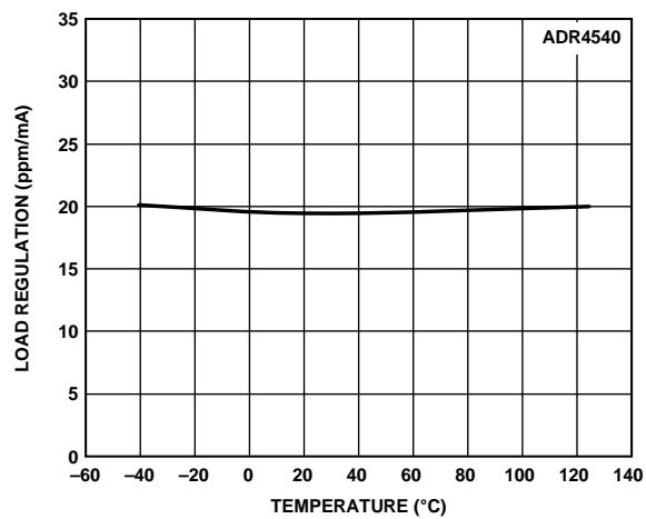
Figure 59. ADR4540 Load Regulation vs. Temperature (Sourcing)
