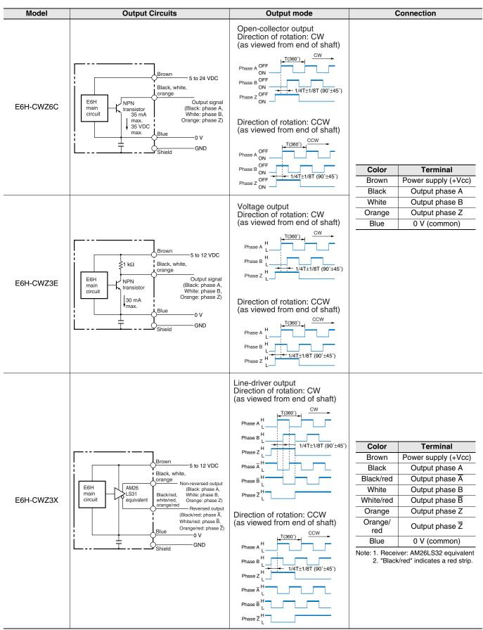
Note: Normally connect GND to 0 V or to an external ground.
